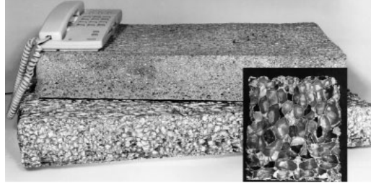
Figure 1.33: Foam samples made by Hydro Aluminium, by blowing gas into SiC containing Al MMCs. Inset: micrograph of similar Alcan type foam [8].
