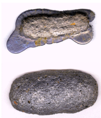
Figure 2.19: Lead foams made from two different lead powders: (at the top) low-oxygen powder (0.06 wt.%) and (at the bottom) higher oxidised powder containing 0.46 wt.% of oxygen [5].
