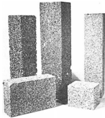
Figure 1.30: Aluminium foam blocks produced in the 1970s by the Ethyl Corp. [8].
