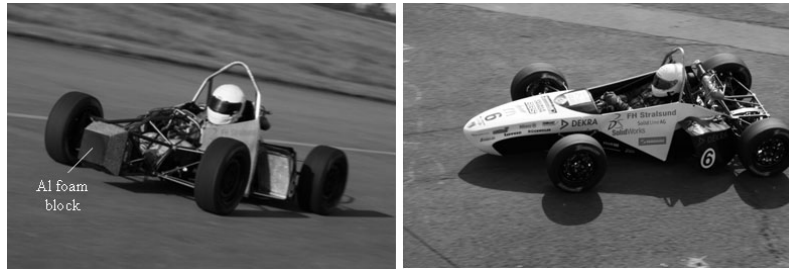
Figure 1.45: Crash protector in a model racing car built by students at the University of Technology of Stralsund, Germany; a. view of car with the front encasement taken off; b. full view [37].
