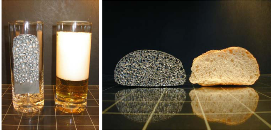
Figure 1.28: On the left: aluminium foam blown with air from a particle-stabilised melt and beer; on the right: zinc foam and bread roll, both foamed by internal gas creation [2]. In the first case, gas is injected continuously to create foam. The foam accumulates to the surface and the result somewhat looks like a glass of draught beer. In the second case, gas-releasing propellants are added to the melt, very similar to the yeast of the baker.
