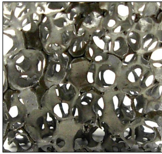
Figure 1.6: An open-cell metal foam (metal sponge) (courtesy of MUSP).
