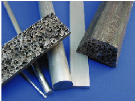
Figure 2.14: Aluminium foamable precursor material (courtesy of MUSP).
