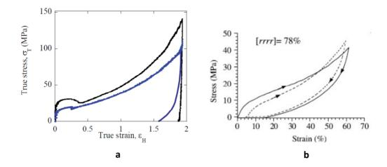
Figure 5. (a)True stress-strain curves of a iPP (black) and s-PP78 (blue). Uniaxial tensile tests performed on dumbbell specimens (gauge length of 33mm) at a constant displacement rate of 5mm/min at T<sub>room</sub>.(b) Nominal stress-strain curves of "plastically" deformed s-PP78 (1° cycle after the plastic deformation process – solid line-; 4° cycle after the plastic deformation process - dotted line -)<sup>1</sup>
