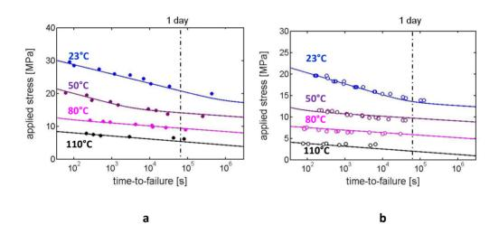
Figure 17. Time to failure prediction (continuous lines) and short term creep experimental data for i-PP\_1 (a) and for i-PP\_2 (b)
