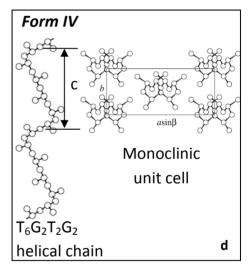
Figure 1. Models of packing of chains in syndiotactic polypropylene <sup>1</sup>
