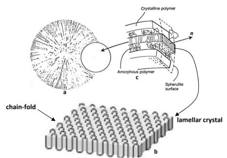
Figure 1. (a) Spherulite composed of lamellar crystals characterized by a chain-folded structure (b) and of the amorphous inter-lamellar phase (c)
