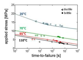
Figure 20. Time to failure prediction (continuous lines) and long-term creep experimental data (data by Sabic) for i-PP 2 including the annealing effect
