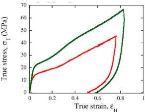
Figure 12. True stress-true strain curves for uniaxial (red line) and plane-strain specimens (areen line)
