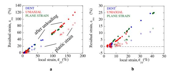
Figure 13. Residual strain component at the end of unloading  $\varepsilon_{res,0}$  (fully symbols) and after the complete recovery of the viscoelastic strain component ,  $\varepsilon_p$  ,(open symbols) versus the applied strain for uniaxial, DEN(T) and plane-strain specimens (a), detail of Figure 13a up to  $\varepsilon_{yy}=8\%$  (b)
