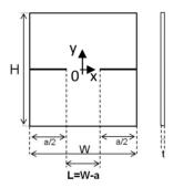
Figure 1. DEN(T) specimen geometry adopted for fracture tests
