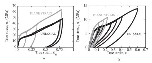
Figure 2: True stress-strain curves relevant to loading-unloading tensile tests performed on uniaxial and plane strain conditions for HDPE (a) and LDPE (b)
