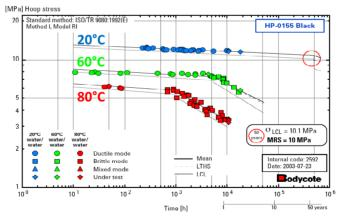
Figure 2. Hoop stress vs. time-to-failure curve built with experimental data of a PE100 at three temperatures (20°C, 60°C, 80°C). A standard method (ISO/TR 9080:1992(E)) was adopted to fit the data <sup>1</sup>
