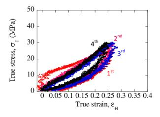
Figure 8b. True stress-strain curves of four subsequent cycles performed on  $R_{1.7}t_{recovery}$ = 7200h
