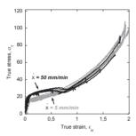
FIGURE 1 Stress/strain curves of sPP
