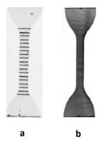
Figure 2. Dumbbell specimens adopted in tensile tests: black lines (a) or an ink pattern (b) were placed on the specimens surface for strain measurement by a video-extensometer or by digital image correlation
