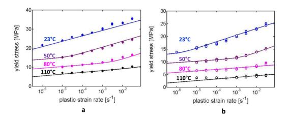
Figure 15. Yield stresses as function of the applied strain rates for i-PP\_1 (a) and for i-PP\_2 (b). The lines are data fitting according to Ree-Eyring equation.
