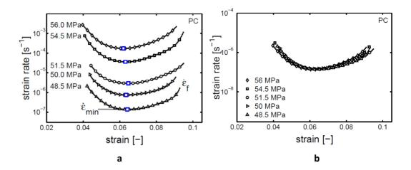
Figure 7. a)Strain rate versus strain by creep tests performed on a polycarbonate at different applied stress levels (Sherby-Dorn plots). b) Sherby-Dorn curves shifted to the curve from 48.5 MPa to illustrate the similarity of the curves
