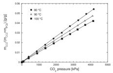
FIGURE 2. Actual sorption isotherms for the PCL/CO2 systems.
