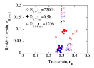
Figure 9a. Residual true strain component versus the applied true strain for all the tested specimens
