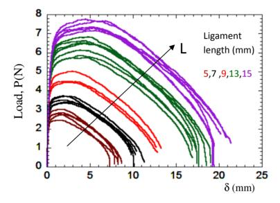
Figure 6. Loading-displacement curves up to specimens fracture of DEN(T) specimens having 5 different ligament lengths (5,7,9,13,15 mm)
