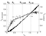
Figure 6: Recovered Hencky strain (○), residual Hencky strain (●) at the end of the unloading vs the applied Hencky strain. The characteristic strains reported in tab.1 are indicated.
