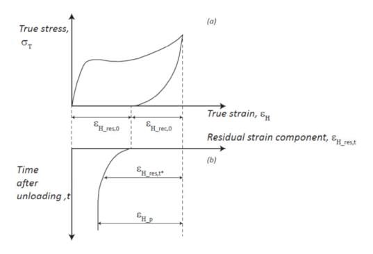
Figure 5. Definition of the residual and recovered strain components of the overall local strain at the end of unloading and in time
