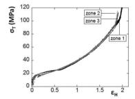
Figure 3: Hencky strain/time curves for three Figure 4: True stress/true strain curves of zones of a single s-PP specimen, in a s-PP monotonic tensile test.
