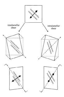
Figure 6. Schematic representation of shear (inter-lamellar slips) and intra-lamella slips (fine and coarse slips) <sup>6</sup>
