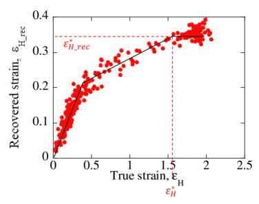
Figure 6. Dependence of the recovered true strain component at the end of unloading on the applied true strain for s-PP78 . Black lines are eyeguide
