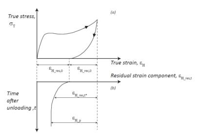
Figure 1: Definition of recovered strain  $(\epsilon_{H\_rec,0})$  and residual strain  $(\epsilon_{H\_res,0})$  components at the end of unloading (a). The plastic strain component  $(\epsilon_{H\_p})$  is also defined (b).
