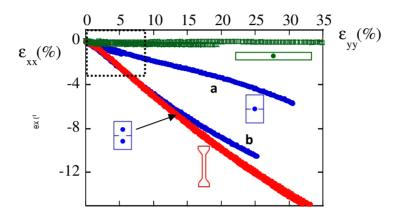
Figure 10. Local strains measured along  $(\varepsilon_{yy})$  and perpendicularly to  $(\varepsilon_{xx})$  the loading direction in the center and at distance of  $\frac{L}{2}$  from the notch plane in a DEN(T) specimen (blue line), along the gauge length of a uniaxial tensile specimen (red line) and in the center of a plane-strain specimen (green line)
