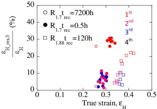
Figure 9b. Percentage of residual true strain component versus the applied true strain for all the tested specimens
