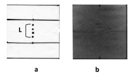
Figure 3. DEN(T) specimens for fracture tests: black markers (a) or an ink pattern (b) were placed on the specimens surface for strain measurement by a video-extensometer or by digital image correlation
