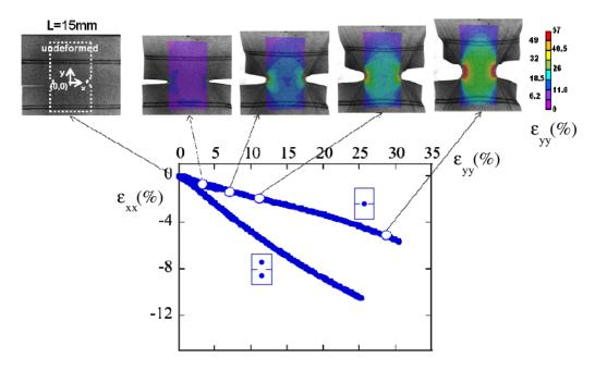
Figure 9. Local strains measured along  $(\varepsilon_{yy})$  and perpendicularly to  $(\varepsilon_{xx})$  the loading direction in the center and at distance of  $\frac{L}{2}$  from the notch plane in a DEN(T) specimen. Strain maps obtained by DIC analysis are also shown in correspondence of different applied strain levels
