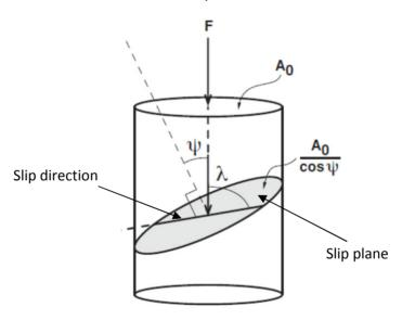
Figure 2. An example of slip direction and of a slip plane along with a crystallographic slip occurs
