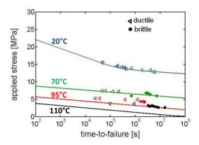
Figure 18. Time to failure prediction (continuous lines) and long- term creep experimental data (data by Sabic) for i-PP\_2
