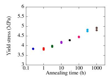
Figure 19. Yield stresses as function of annealing times (h) on a semilogarithmic scale for i-PP\_2. Data relevant to uniaxial tensile tests performed at  $\varepsilon=10^{-3}s^{-1}$  and at T=110°C.
