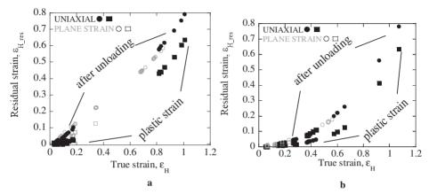
Figure 3: Dependence of the residual strain at the end of the unloading,  $\epsilon_{H\_res,0}$ , and after the recovery of the viscoelastic strain component –  $\epsilon_{H\_p}$  – on the applied strain for HDPE (a) and LDPE (b).
