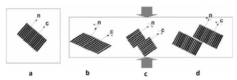
Figure 4. Rotation of the chain axis,  $\underline{c}$  and of the axis normal to lamella  $\underline{n}$  produced by fine slip (b), coarse slip (c) and inter-lamellar shear (d). In (a) orientation of both vectors in lamella prior to deformation is shown <sup>1</sup>
