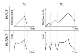
**FIGURE 2** Sketch of a single-cycle (a) and multi-cycles (b) loading-unloading tensile tests.
