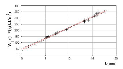
Figure 7. Specific fracture energy  $w_f$  (experimental data – black symbols) versus the ligament length for all the tested samples; Linear fit of the experimental data (red line) is also reported
