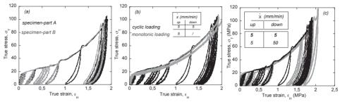
FIGURE 3 True stress/true strain curves for multi-cycles test (a) compared to those related to monotonic test (b) (displacement rate of 5 mm/min for the loading and unloading steps), (c) multi cycles tests at different unloading displacement rates.
