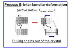
Figure 16. Schematic representation of the molecular mechanisms involved in processes I and II <sup>4</sup>
