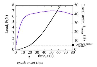
Figure 8. Load curve (purple line) and local strain in the central zone of the ligament plane (black line) as function of time; the time at crack onset and the strain at crack onset are also reported
