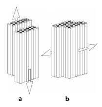
Figure 3. Two types of crystallographic slip in macromolecular crystals: (a) longitudinal slip (b) transversal slip<sup>1</sup>
