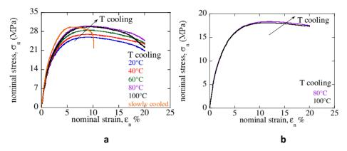
Figure 10. Nominal stress-strain curves of i-PP\_1 (a) and i-PP\_2 (b) cooled down to different temperatures; tests performed at  $\varepsilon = 10^{-3} s^{-1}$  and at  $T_{room}$ .
