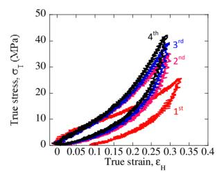
Figure 8a. True stress-strain curves of four subsequent cycles performed on  $R_{1.7}t_{recovery}$ = 0.5h
