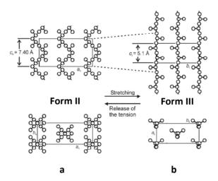
Figure 2. Reversible crystal-crystal transition between form II (a), stable after unloading , and form III (b), stable at high applied strains
