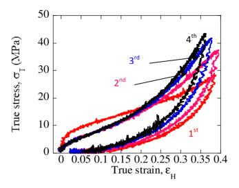
Figure 8c. True stress-strain curves of four subsequent cycles performed on  $R_{1.88} t_{recovery}$ = 120h
