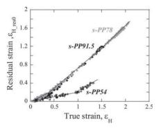
**FIGURE 10** Dependence of the residual strain component on the applied true strain for s-PP54, s-PP78, and s-PP91.5.
