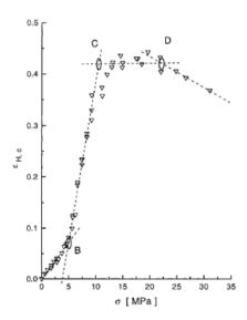
Figure 8. Applied (step cycle), recovered (cyclic) and residual (basic)strains as function of the applied true stress. Data relevant to loading-unloading tensile tests performed on a PEVA12. Points
