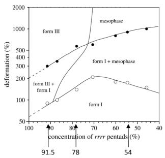
Figure 3. Strain values at the onset (open cyrcle) and at the end (full cyrcle) of the form I -> form III transformation as a function of [rrrr] pentad content 16
