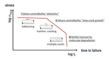
Figure 1. Schematic representation of a hoop stress vs. time-to-failure curve with the illustrations of failure mechanisms
