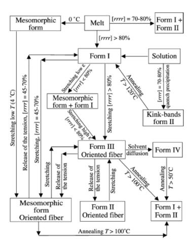
Figure 4. A scheme of the crystal form transitions observed in s-PP induced by annealing or straining <sup>1</sup>
