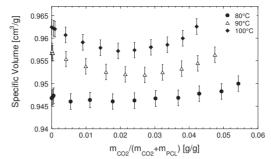
FIGURE 4. Specific volume of the solution PCL/CO<sub>2</sub> as a function of CO<sub>2</sub> mass fraction. Error bars evaluated by accounting for the error propagation in the whole measurement chain.
