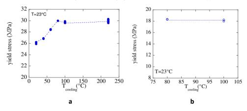
Figure 11. Yield stress versus  $T_{cooling}$  for i-PP\_1 (a) and i-PP\_2 (b) cooled down to different temperatures. Data are relevant to uniaxial tensile tests performed on i-PP\_1 and i-PP\_2 at  $\varepsilon=10^{-3}s^{-1}$  and at  $T_{room}$
