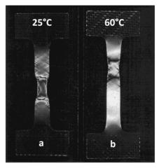
Figure 5. Images of dumbbell specimens of quenched isotactic polypropylene drawn at 25°C (a) and at 60°C (b) up to  $\varepsilon_N = 0.3$  ( $\dot{\varepsilon} = 1.05*10^{-3} s^{-1}$  crossed polarizers)<sup>4</sup> (See text)
