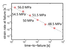
Figure 6. Strain rate at failure versus the time-to-failure from creep tests on a polycarbonate 4
