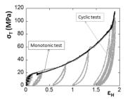
Figure 5: True stress/true strain curves for multi-cycles test (grey line) compared to those related to monotonic test (black line)
