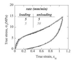
FIGURE 7 True stress-strain curves of s-PP54 in two single-cycle tests unloaded at different displacement rates.
