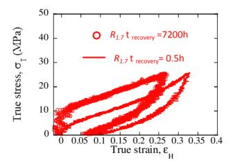
Figure 7. True stress-strain curves (1<sup>st</sup> cycle) relevant to samples  $R_{1.7}$   $t_{recovery}$ = 0.5h (solid line) and  $R_{1.7}$   $t_{recovery}$ =7200h (open symbols)
