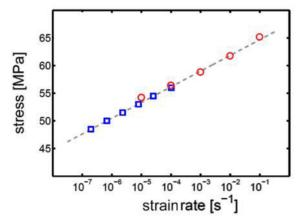
Figure 8. Relation between the stresses and the applied strain rates in constant strain rate tests (red symbols) and between the applied stresses and the secondary creep strain rates in creep tests (blue symbols) 4
