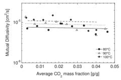
FIGURE 3. Mutual Diffusivity for the PCL/CO<sub>2</sub> solution as a function of CO<sub>2</sub> concentration.
