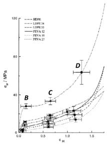
Figure 10. True stress-strain curves for three different polyethylenes and polyethylenvinilacetates differing in their crystallinity degree. The characteristic points B-D are reported <sup>6</sup>
