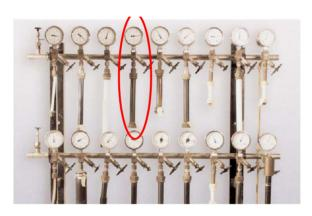
Figure 3. Hostalen GM 5010 pipes under constant pressure since 1956
