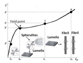
Figure 1: True stress-true strain curve for a semicrystalline polyolephine with microstructural changes occurring during the tensile test [4]
