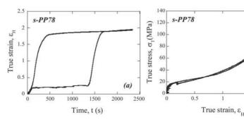
FIGURE 4 True strain vs. loading time measured in two different zones of a single s-PP78 dumb-bell specimen (a) and the relevant true stress-strain curves (b). Displacement rate 5 mm/min.
