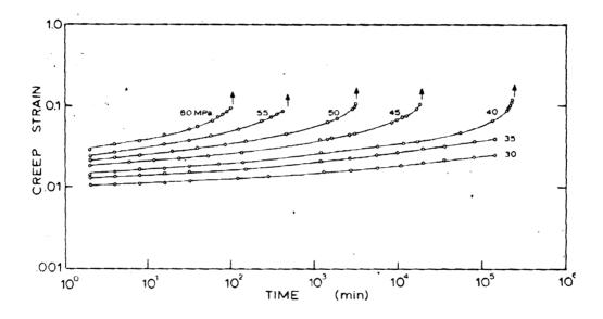
Figure 5. Creep strain versus time for PMMA aged at  $T_{room}$  for over 5 years at different applied engineering stresses (T=22.5°C)<sup>10</sup>
