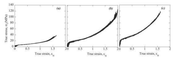
FIGURE 6 True stress-strain curves for s-PP54 (a), s-PP78 (b), and s-PP91.5 (c). Displacement rate 5 mm/min.
