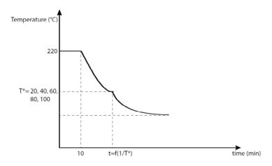
Figure 9. Schematic graph reporting the conditions (time, temperature) of the cooling process adopted in the compression molding process for i-PP\_1 and i-PP\_2 at TU/e
