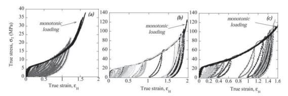
**FIGURE 8** True stress-strain curves in monotonic loading and multi-cycles loading-unloading tests for s-PP54 (a), s-PP78 (b), and s-PP91.5 (c). Loading and unloading at 5 mm/min.
