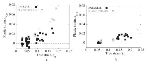
Figure 4: Detail of Figure 3.(a) Data relevant to HDPE (b) data relevant to LDPE.
