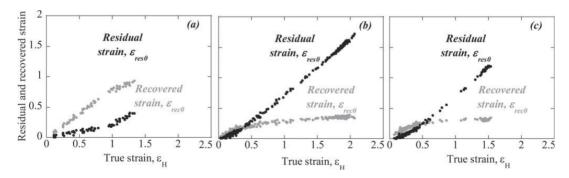
FIGURE 9 Dependence of the residual and recovered true strain components on the applied true strain for s-PP54 (a), s-PP78 (b), and s-PP91.5 (c).
