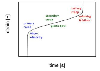
Figure 4. Schematic representation of a strain vs. time curve obtained by a creep test.
