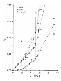
Figure 7. Applied (step cycle), recovered (cyclic) and residual (basic) strains as function of the applied true stress. Data relevant to loading-unloading tensile tests performed on a PEVA12.
