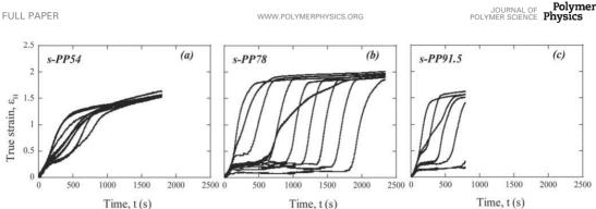
FIGURE 5 Time dependence of the true strain measured in different zones of a single specimen of s-PP54 (a), s-PP78 (b), and s-PP91.5 (c). Displacement rate 5 mm/min.
