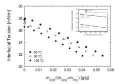
FIGURE 5. Effect of CO<sub>2</sub> concentration on the interfacial tension of PCL in CO<sub>2</sub>. Inset: Effect of temperature on the interfacial tension of the solution PCL/CO<sub>2</sub> as a function of CO<sub>2</sub> mass fraction.
