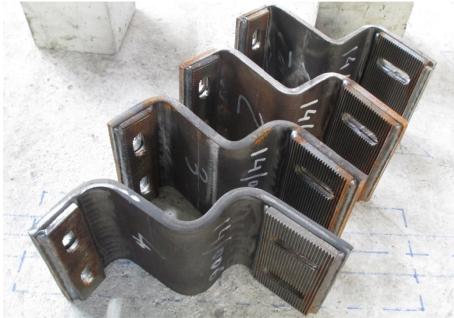
Figure 3.71 – Folded plates specimens before testing
