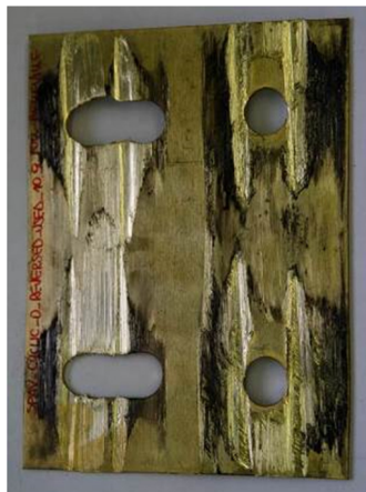
Figure 3.20 – Brass sheet after testing with protocol E
