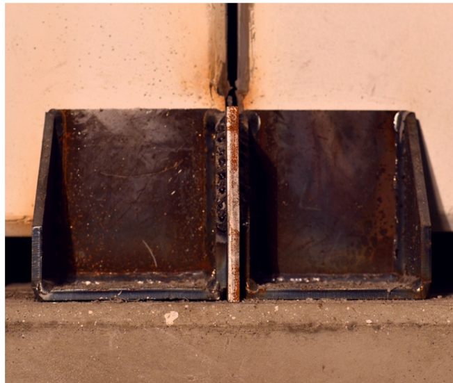
Figure 5.42 – Out-of-plane retainer and in-plane stopper device for rocking configurations
