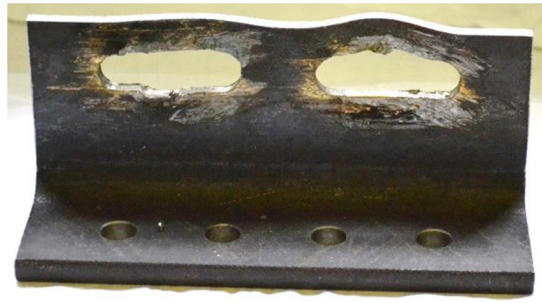
Figure 3.12 – Strong plastic deformation of the T-shaped support profile after tangling
