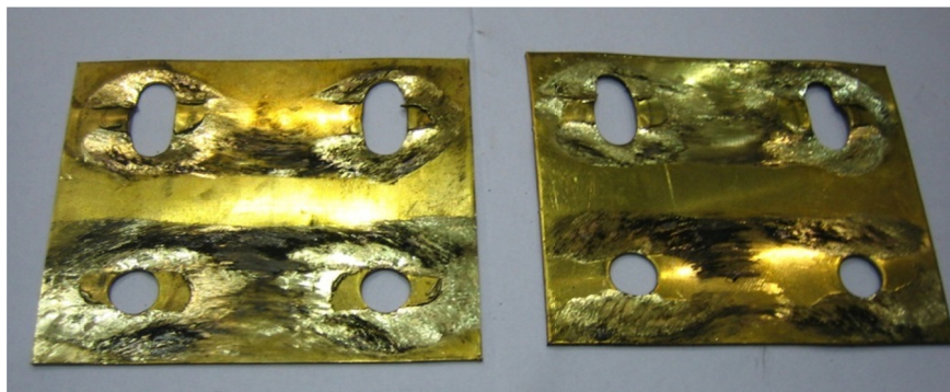
Figure 5.77 – FBD brass plates after the whole series of tests on dissipative systems
