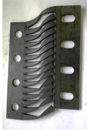
Figure 4.29 – MSD plate after the test
