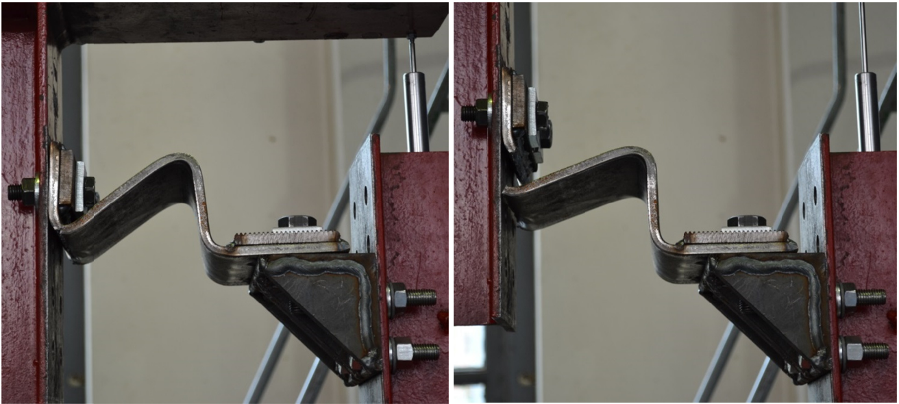
Fracture initiation at 70 mm downwards displacement
