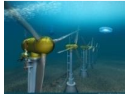
Figure 1-7 Tidal current axial turbines
