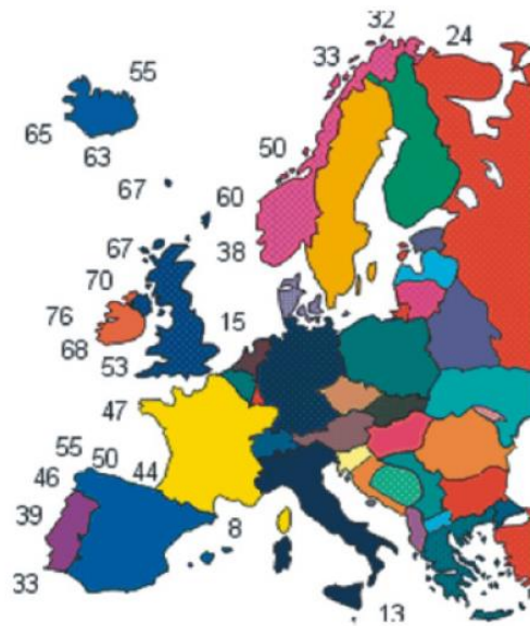
Figure 1-10 Power distribution at the European level (kW/m)
