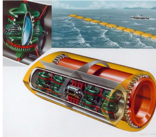
Figure 1-24 Salter's Duck buoy
