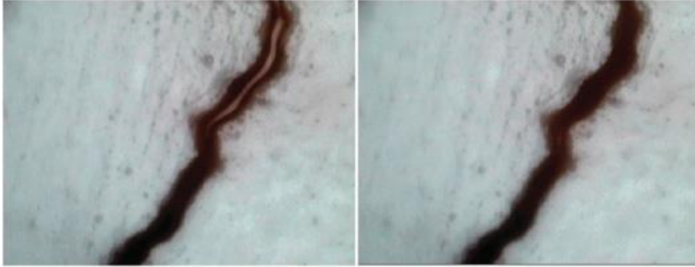
Figure 1.15: Microscope photos of self-healing coating films with urea–formaldehyde microcapsules immediately after crack formation (left) and after 90 s (right) 50 .
