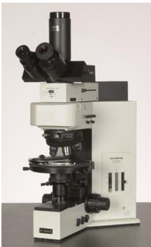
Figure 2.20: Olympus BX-60 optical microscope utilized to carry out visual analyses on samples.
