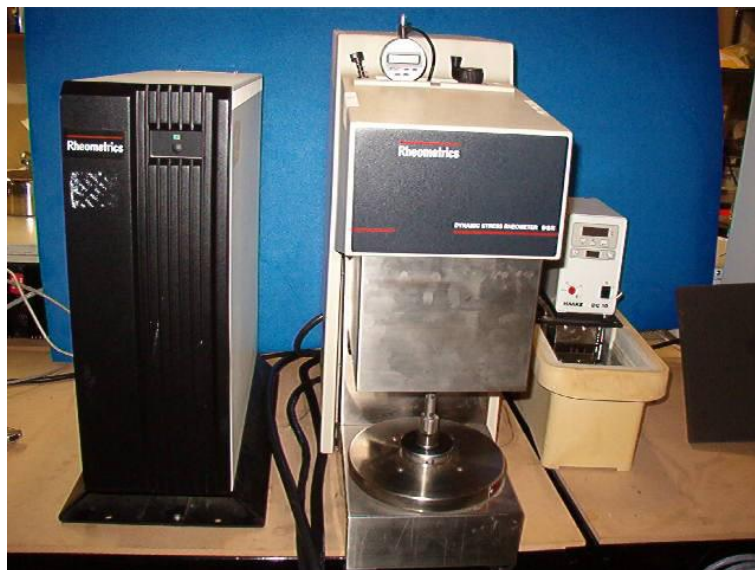
Figure 2.24: Rheometrics DSR200 instrument utilized to carry out rheological analyses.
