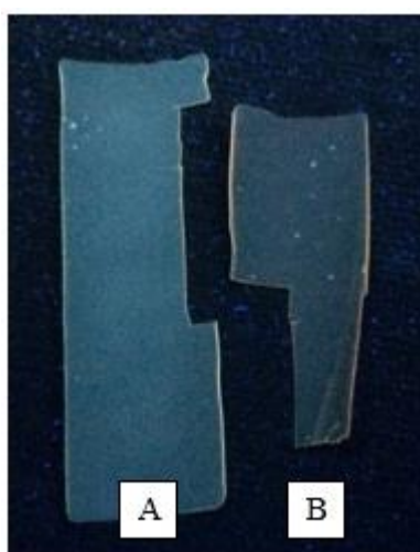
Figure 2.15: synthetized polyurea films (a) ACBP amine based (b) DABP amine based under UV-irradiation at 366nm.
