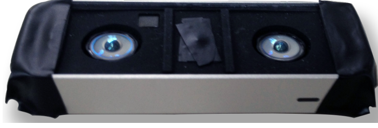
Figure 4.6. Leap Motion: the LeapMotion is disassembled and the LEDs are covered with black insulating tape.
