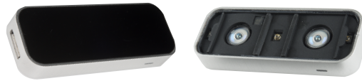
Figure 4.1. LeapMotion: the LeapMotion device. On the right the black cover plate is removed to show the three IR LEDs and the two lenses.
