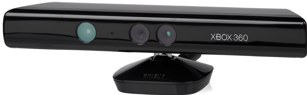
Figure 4.3. Kinect: the Kinect device. The leftmost lens covers the IR projector. The other two lenses are an IR sensor and a standard camera but will not be used in the proposed acquisition system.
