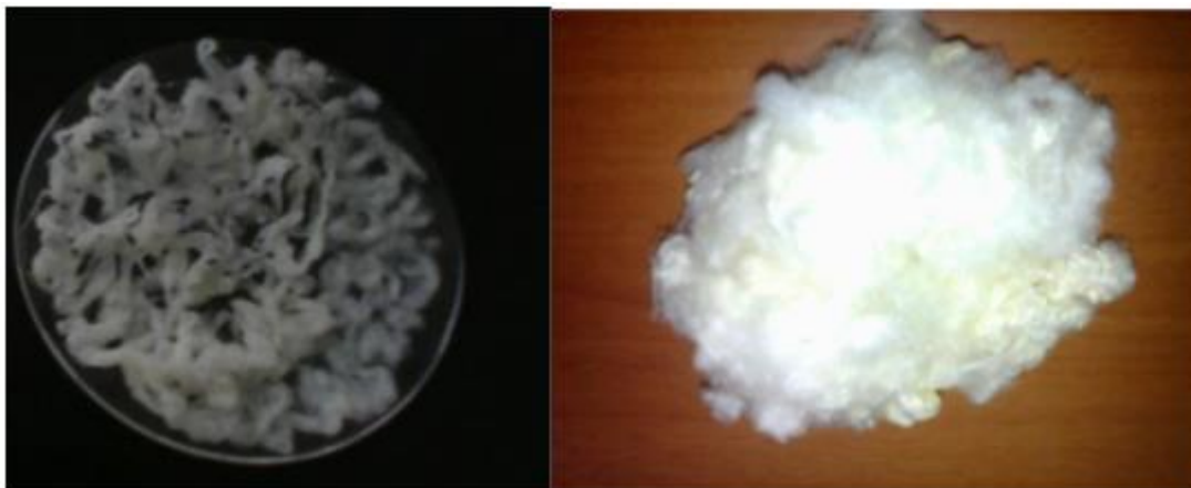
Figure 5.1 Silk immediately after degumming (left), dried silk (right)
