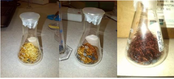
Figure 1. Silk fiber during iodine vapor treatment. After 3 hours (left), after 5 hours (middle), after 26 hours (24 hours at room T and another 2 hours at 70° inside a woven) (right).
