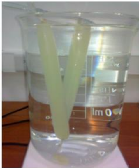
Figure 5.2 Dialysis of the aqueous silk fibroin with distilled water.
