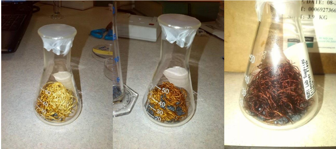
Figure 3.1. Silk fiber during iodine vapor treatment. After 3 hours (left), after 5 hours (middle), after 26 hours (24 hours at room T and another 2 hours at 70° inside a woven) (right).
