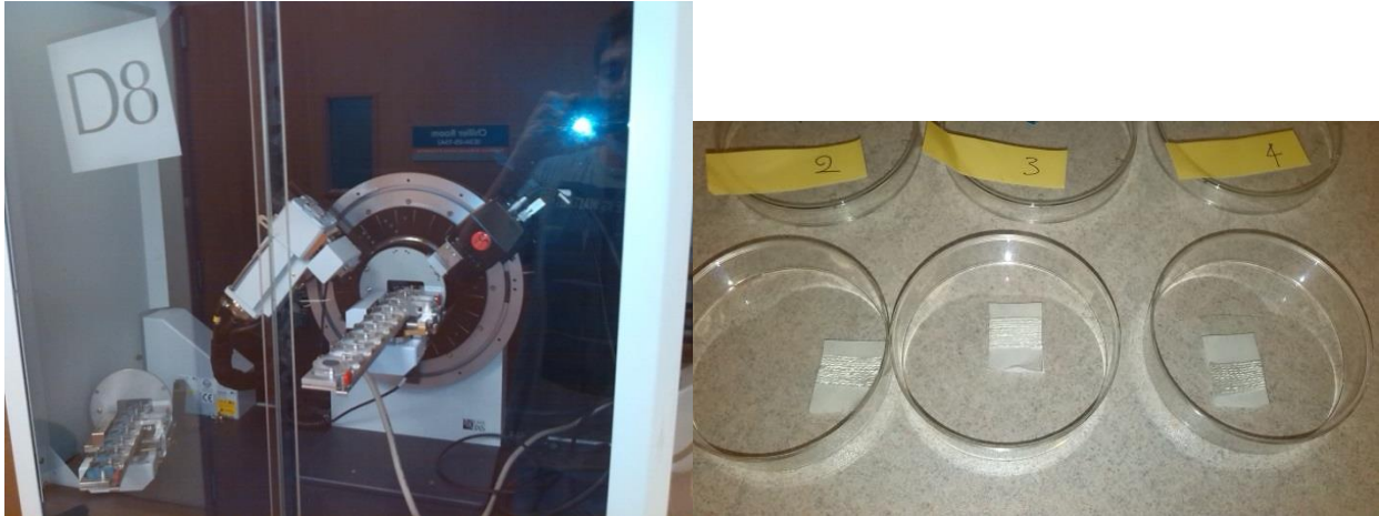
Figure 2.8: Bragg Brentano diffractometer at NUS laboratory (Singapore) (left). Sample preparation before XRD analysis (right).
