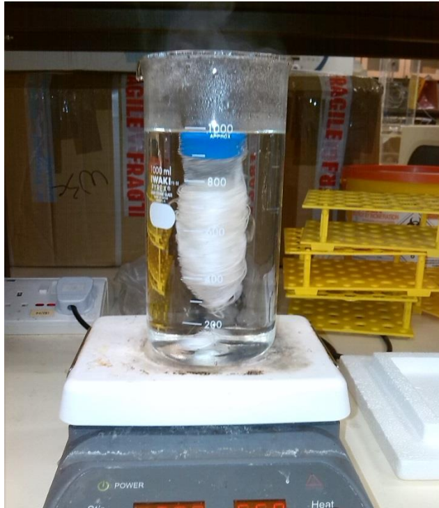
Figure 3.2. Silk hunk rolled to a plastic container during KBr treatment
