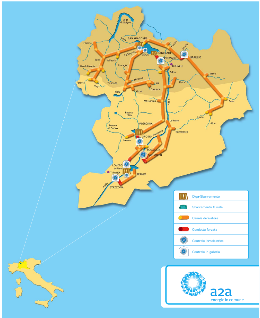
Figure 3.3: A2A hydropower network in Valtellina, adapted from A2A
