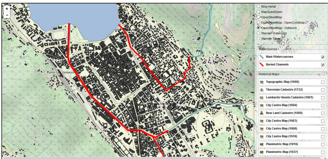
Figure 61: WebGIS displaying the buried channel paths.
