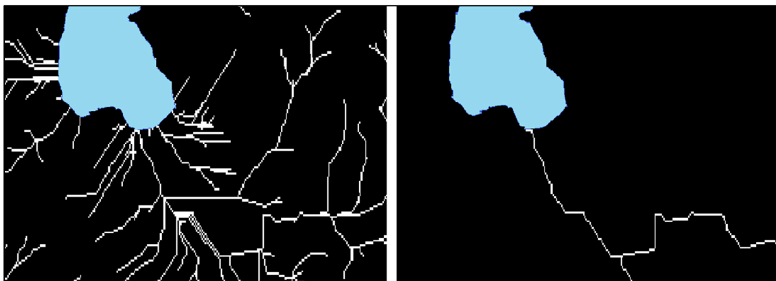
Figure 17: Flow Accumulation raster (computed from HeliDEM) dipped over Como V alley. The white lines represent the flow-paths for two different classification break values: 100(left) and 5,000(right) upstream flow cells. In the first case the catchment area of any visible stream is \geq 0.04 \text{ km}^2 while, in the second case, it is \geq 2 \text{ km}^2 .
