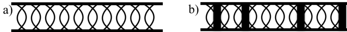
Figure 3.8: Stylized representation of Hybrix™ core structure with proper separation of the metal facing (a), with local region of through-thickness epoxy adhesive (b)
