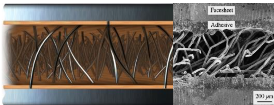
Figure 2.1: Hybrix™ cross-section showing the different constituents: i.e. metal facing, adhesive layer ad polyamide 6,6 fibres
