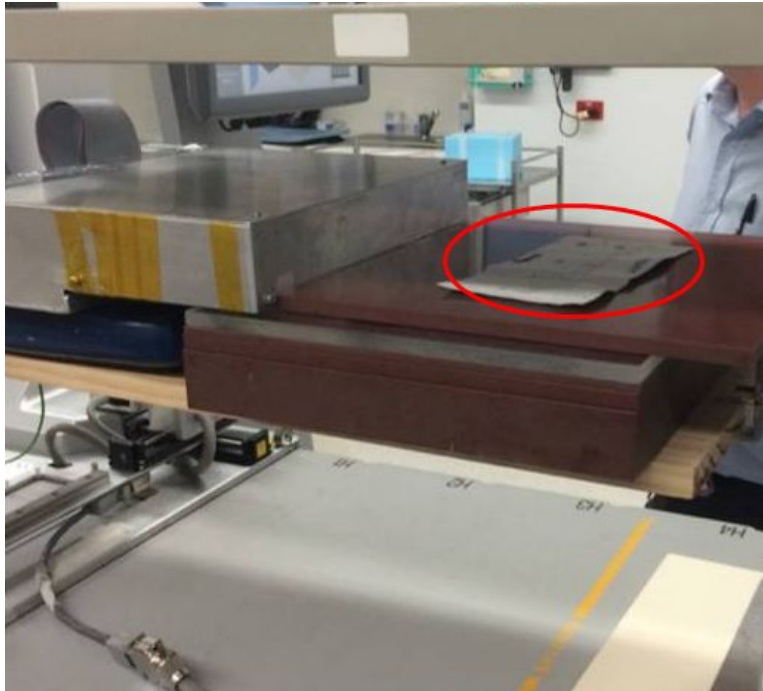
Figure 4.4: The beacons are placed on a white paper as shown in Figure 1.3 and placed over the detector.
