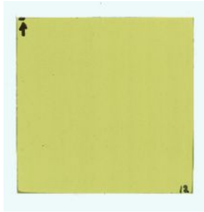
Figure 3.2: One 10x10mm 2 film sample. The serial number 12 and the orientation arrow are visible.
