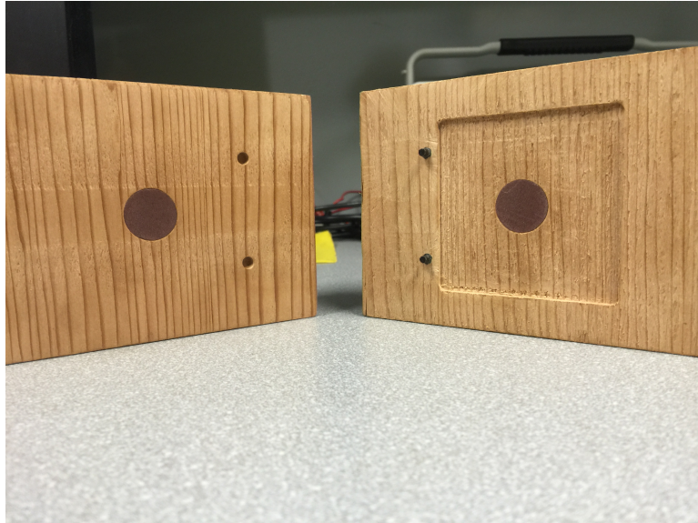
Figure 7.1: New timber pieces: they feature two solid water hemispheres representing the tumour.
