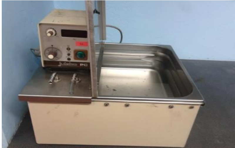
Figure 3.7: Julabo 12-b oil-bath
