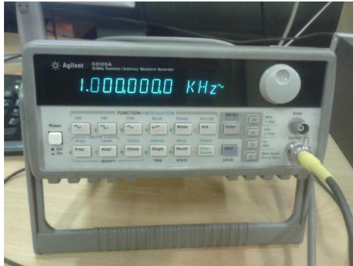
Figure 4.3: The frequency generator is used to produce signal of known shape and frequency
