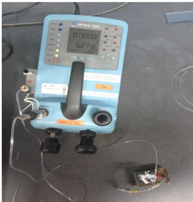
Figure 3.23: Setup for the calibration of the SENSYM (differential pressure transducer)
