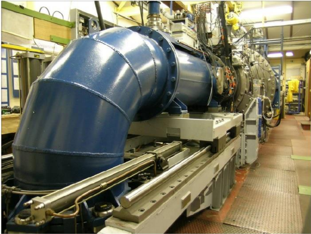
Figure 2.1: The turbine test rig of Von Karman Institute
