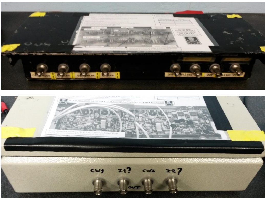
Figure 3.22: The cold wire boxes (Wheatstone bridge)
