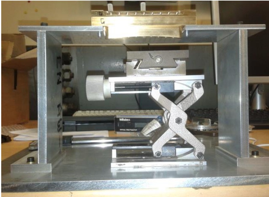
Figure 2.5: The metallic tool designed in CATIA; in the bottom a picture of the setup used to set the correct position and angle of the probe.
