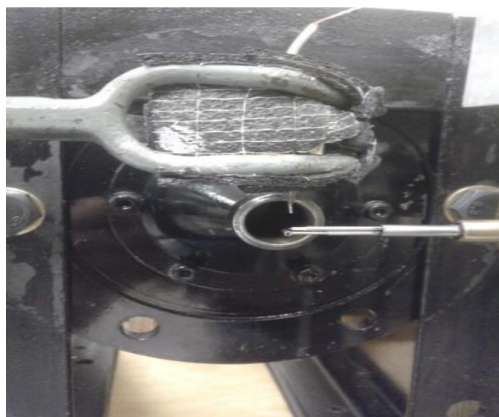
Figure 3.25: Thermocouple 4R (up) and cold wire (put horizontally).
