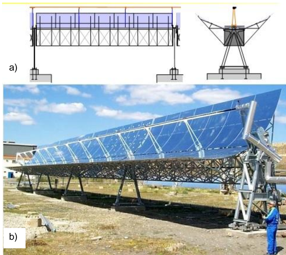
Figure 4-2 Euro-Trough system: a) Supporting structure sketch, b) Test facility (Lupfert et al, 2001).
