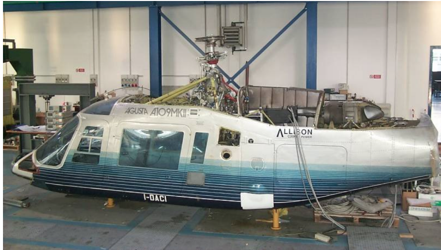
FIGURE 2.1: Helicopter fuselage mock-up employed in the Friendcopter project.
