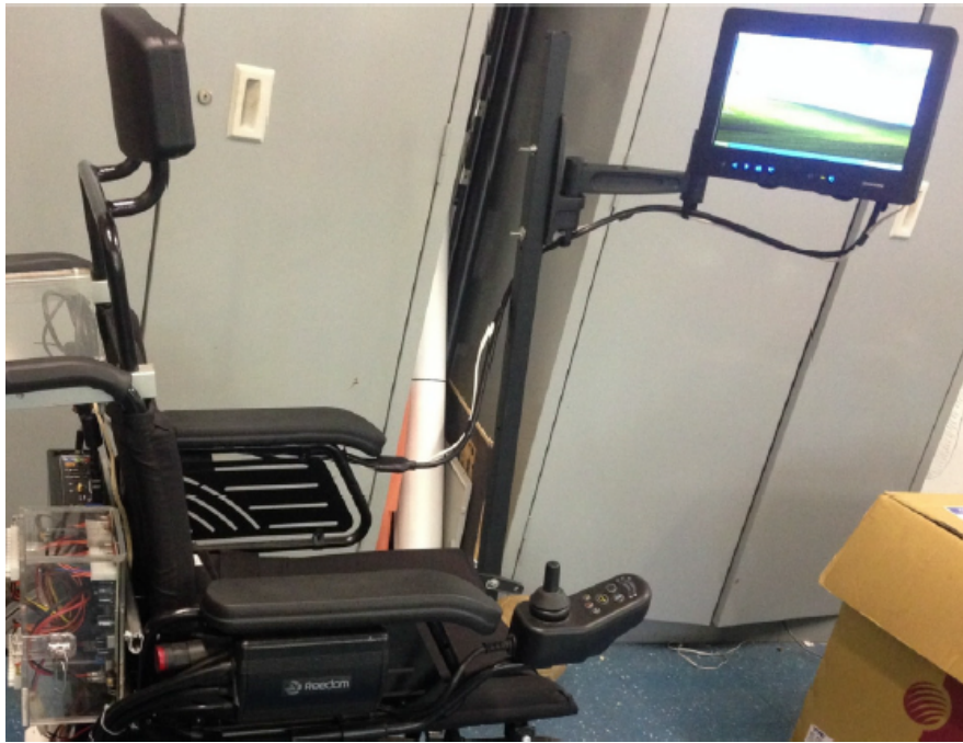
FIGURE 3.2: UFES robotic wheelchair. The Freedom wheelchair has been equipped with a computer behind the seat and a touchscreen monitor mounted on an aluminum structure.
