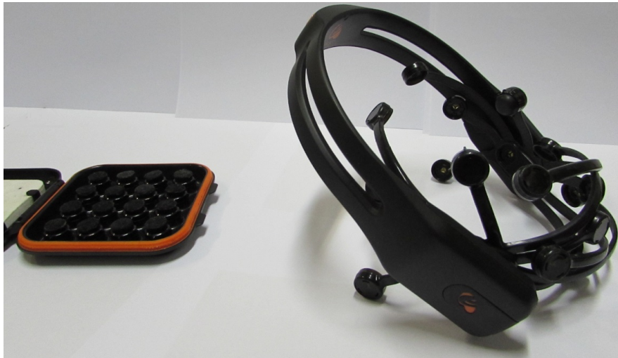
FIGURE 5.1: Emotiv EPOC headset. On the left, the electrodes inside the hydration box.
