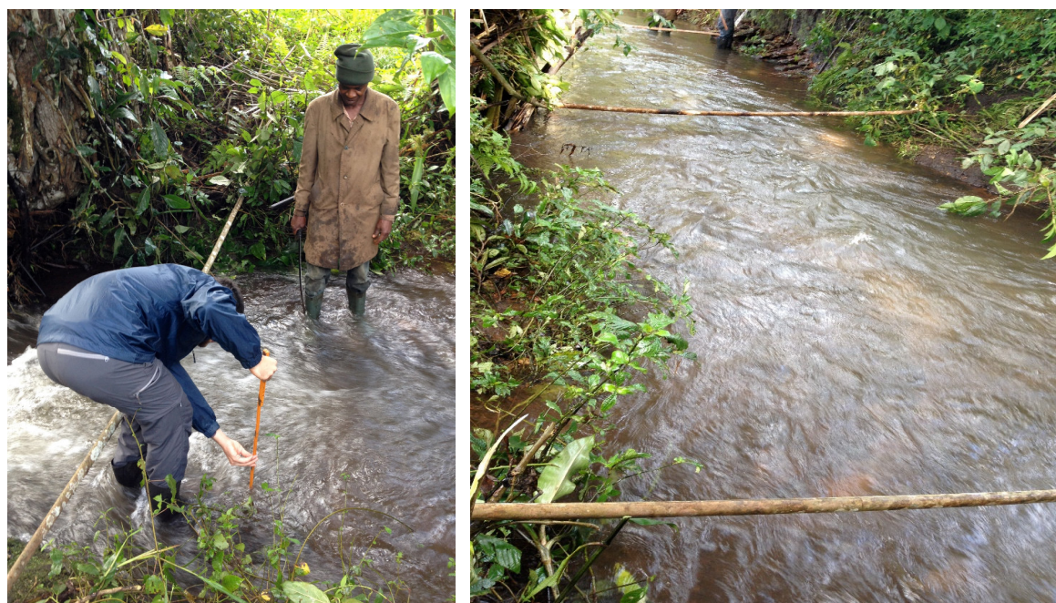
Figure 2.6 Depth measurement (left); 10m distance of the stream (right). Source: Authors
