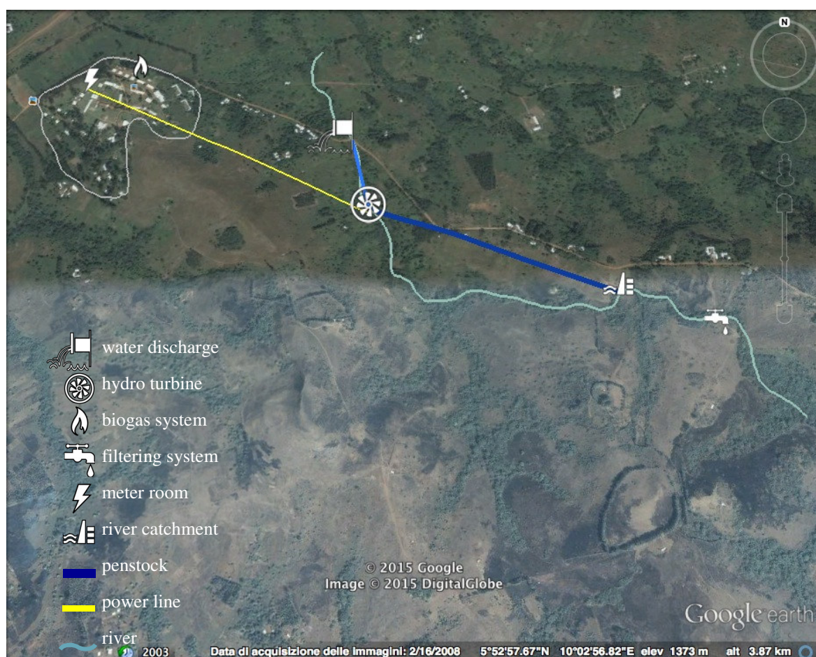
Figure 2.8 Proposed layout of Micro hydropower scheme. Source: adapted by authors from Google Earth
