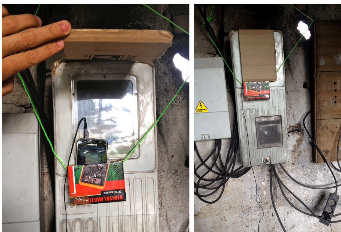
Figure 2.5 Set up of smartphone for load profile measurements. Source: Authors
