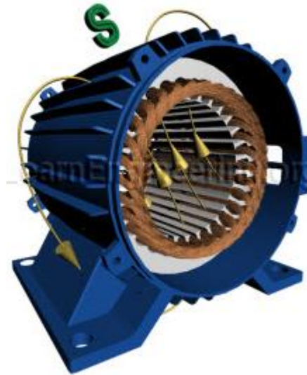
Figure 2: Rotating Magnetic Field Produced in an Induction Motor
