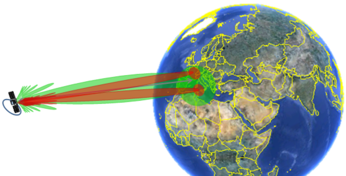
Figure 2.1: GEOSAR system; L-band (green ray), X-band (red rays)
