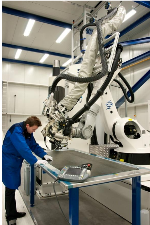
Figure 2-7: DAFP using AFP with dry fiber tapes at NLR. (Source: www.nlr.nl )
