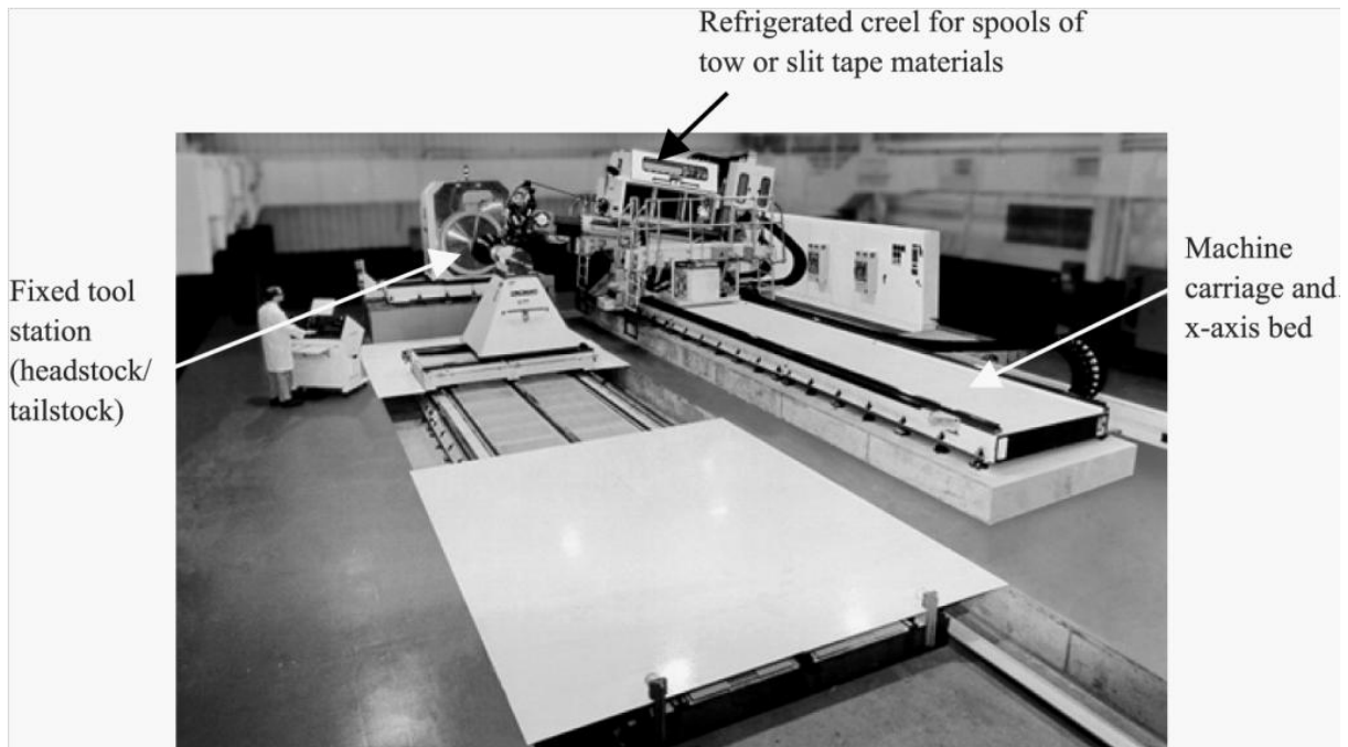
Figure 1-11: Typical FP machine configuration (Cincinnati Machine Viper 3000) [1]
