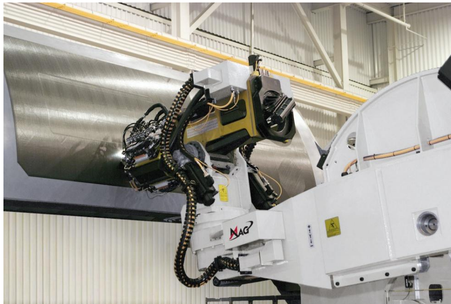
Figure 1-12: Fiber placement head. (Source: www.mag-ias.com )
