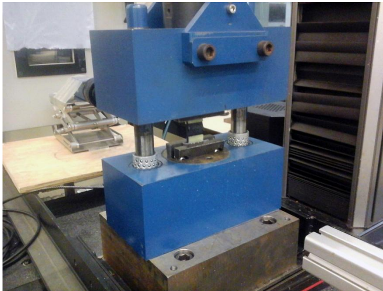
Figure 5-3: Compression specimen in the test fixture
