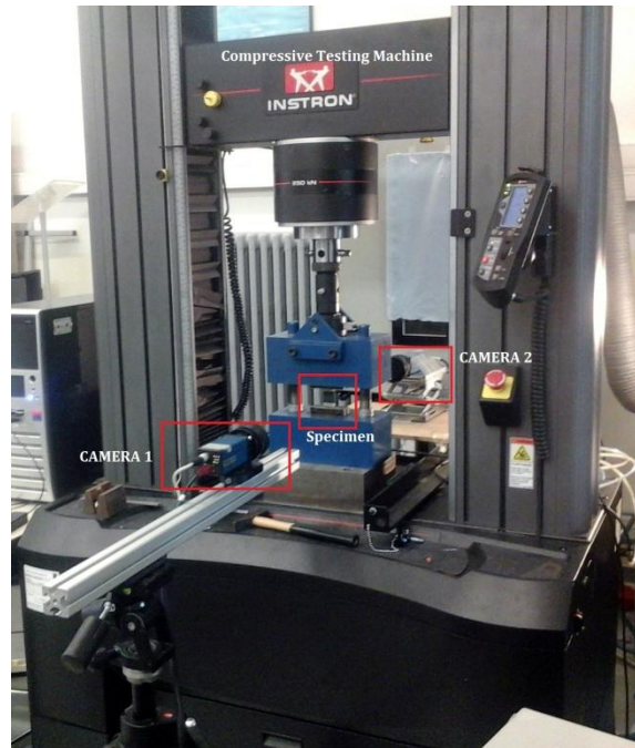
Figure 5-4: Back-to-back strain measurement
