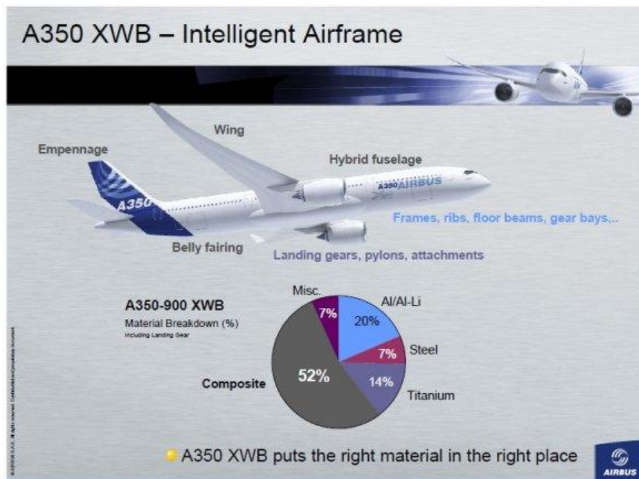
Figure 1-1: Airbus A350XWB airframe. (Source: aerospace.honeywell.com)
