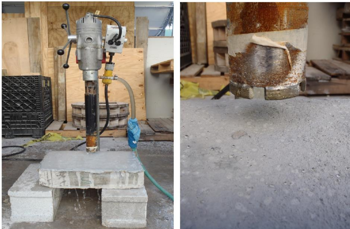
Figure 2. 17 - Core drill to cut the specimens, Bianchi et al. (2013)
