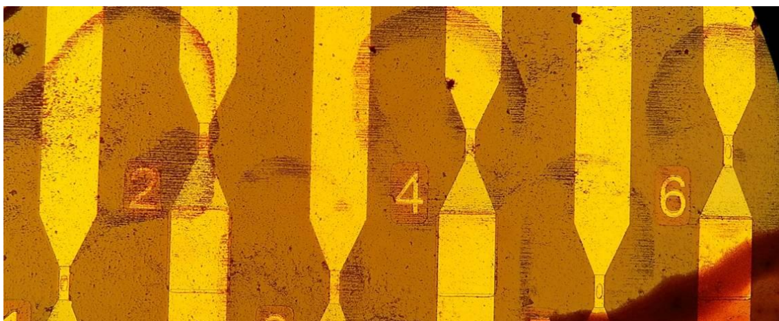
Figure 5.2 Optical image of the functionalized sensors after the biological experiment. The analyte is uniformly distributed over the spotted area.
