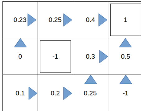
Figure 2.2: Example of value function used in a critic-only method for a discrete model and the derived optimal policy (arrows).
