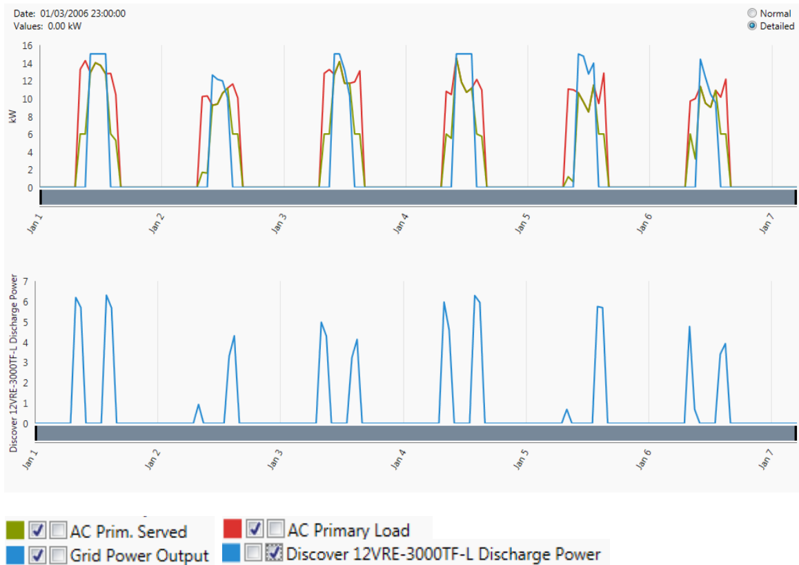
Fig. 5.26: Trend of energy load, energy load served, grid power output and batteries state of charge
