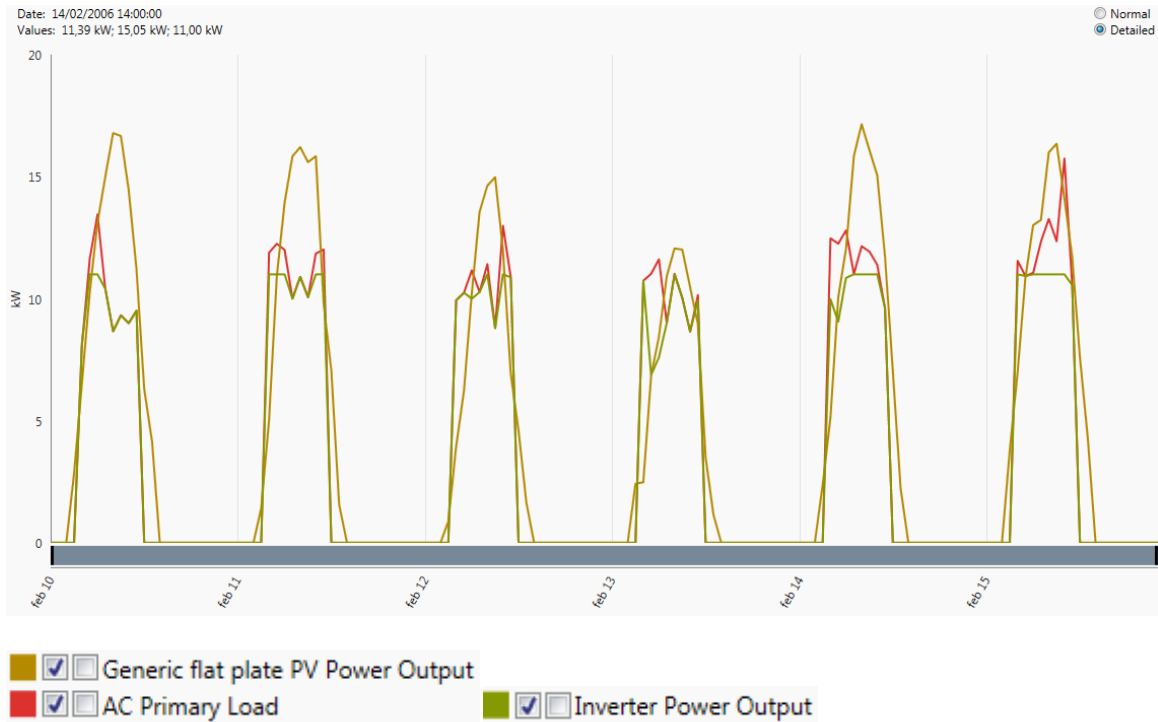
Fig. 5.24: Trend of energy load, solar PV output and inverter power output
