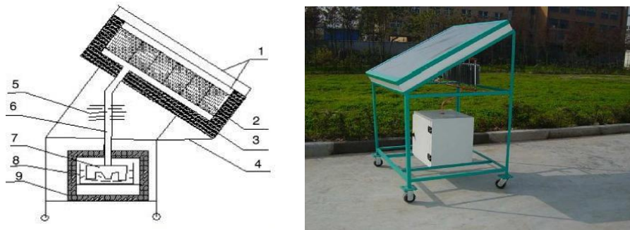
Figure 2-19 The schematic and a photograph of the solar icemaker [25]
