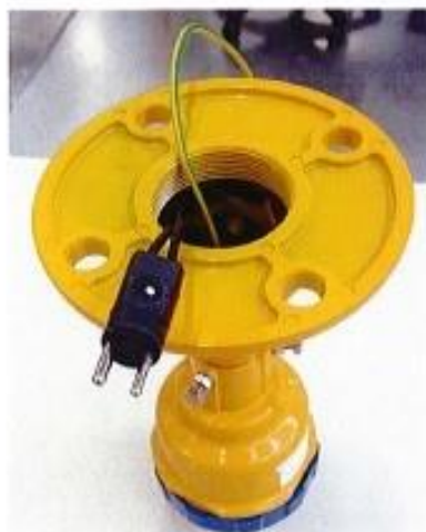
Figure 43 LETE sample for the test of degree of protection
