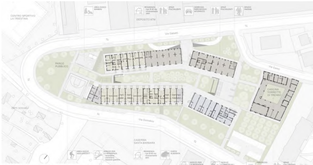
Figure 8-57 Ground floor plan of social housing in via Cenni (source from http://www.cennidicambiamento.it )
