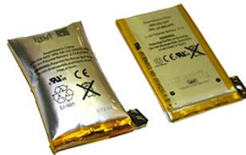
Figure B.11 Example of the variation in volume of a pouch cell during the charging/discharging cycle. [70]
