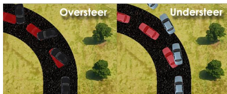
Figure 3.5 Example of an oversteering (left) and understeering (right) behaviour of a car. [30]
