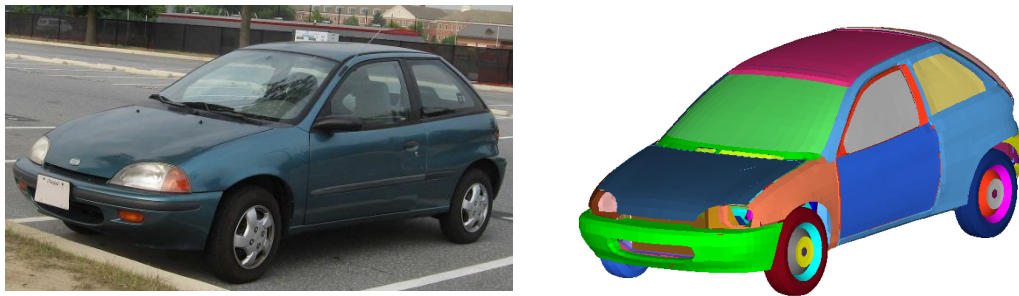
Figure 4.1 Comparison between the Geo Metro (left) [38] and the FE model of the vehicle (right) [37].
