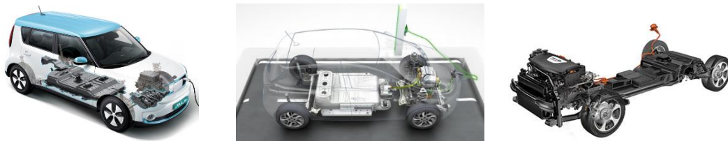
Figure 5.8 Examples of three EVs in the current market that use the tunnel zone and the area under the front seats for the integration of the batteries. From the left: Kia Soul electric 2015 model [46], Renault Zoe 2014 model [47] and Fiat 500 E 2014 model [48].
