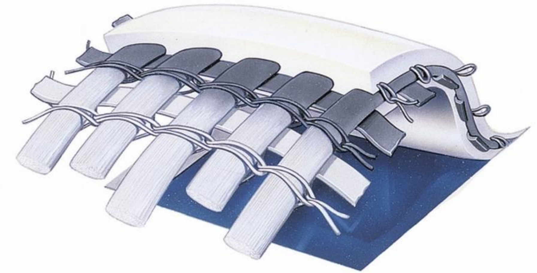
Figure 96) A woven polyester base fabric with vinyl coating
