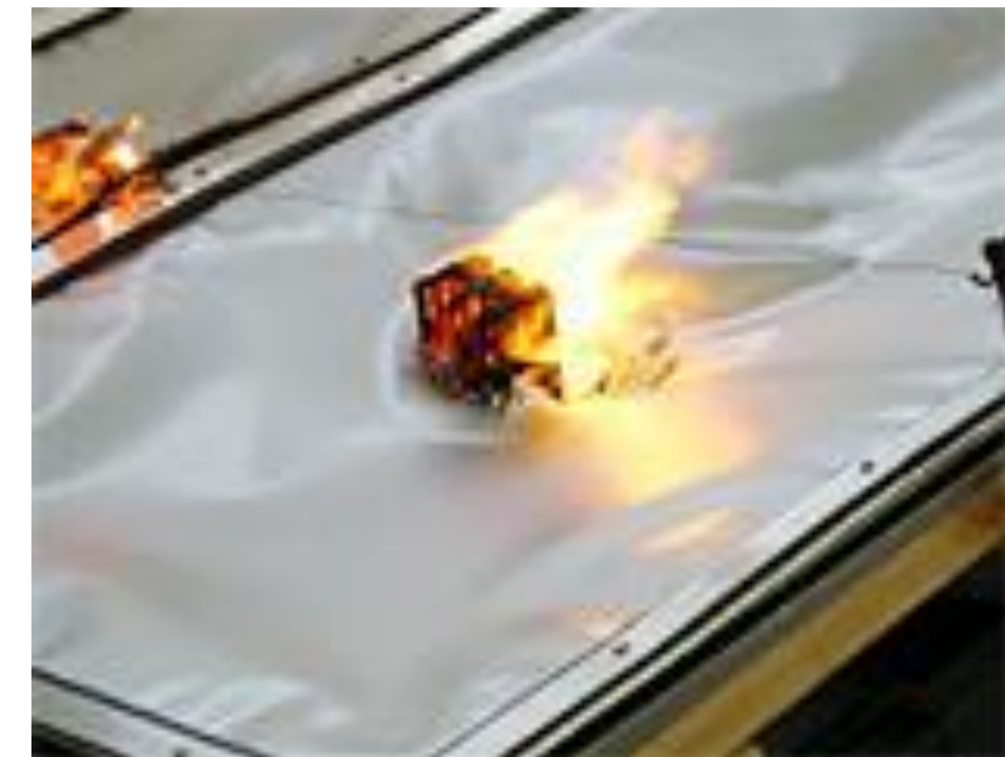
Figure 133) Fire resistant Class 1 in Italy and B1 in Germany
