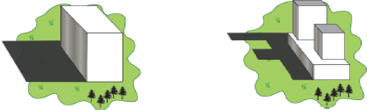
Figure 39 Mitigation of shadow impact; BEFORE (left) and AFTER (right)
