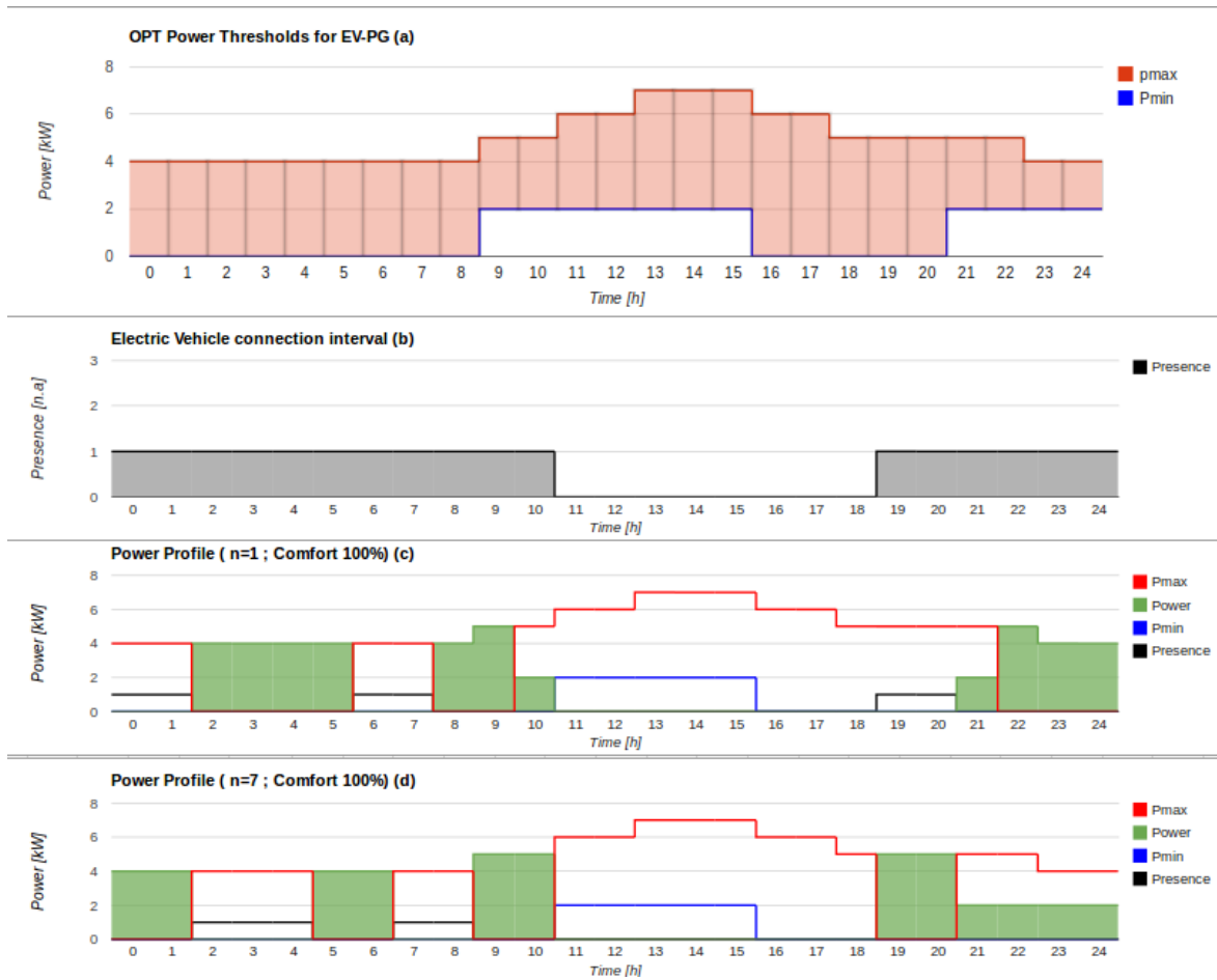
Figure 6.8: General sequence of profiles managed by the EV-PG during an optimization process. Timeslot = 60 min. Profile (a) reports the thresholds received from the Optimizer, (b) is the presence profile of the vehicle connected to the WallBox according
