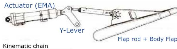
**Figure 6.3:** Flap Control System (Courtesy of Thales Alenia Space Italia)
