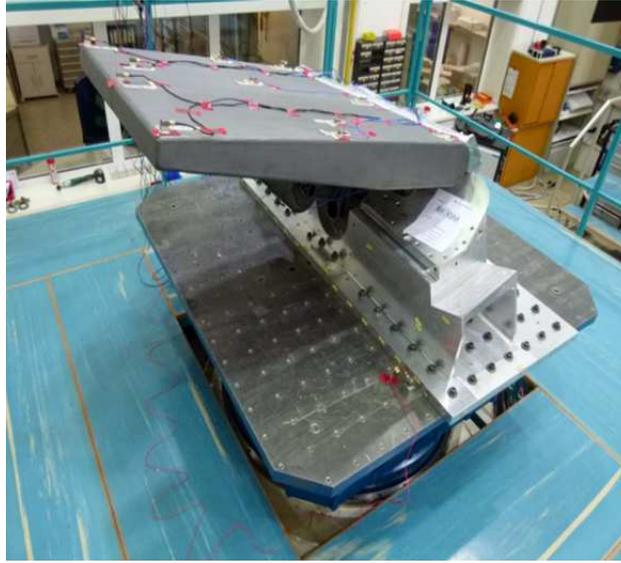
**Figure 6.4:** Flap testing set-up (Courtesy of Thales Alenia Space Italia)
