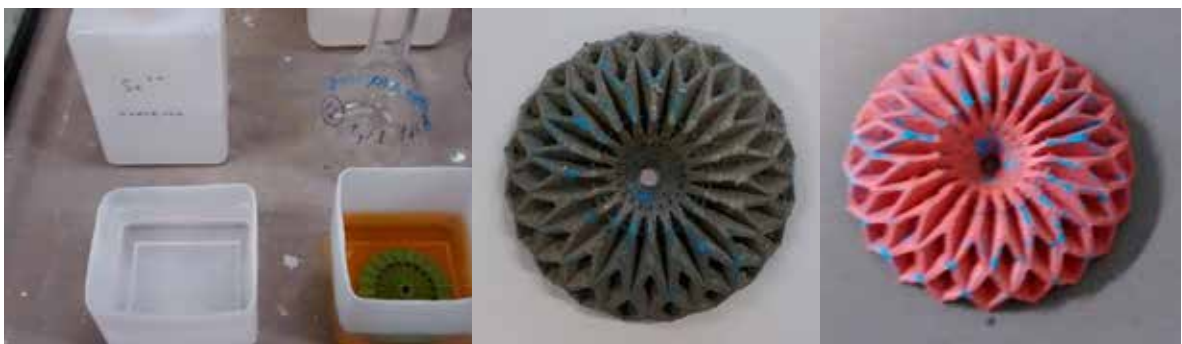
Figure 89: PLA copper plating tests at Politecnico di Milano. Acid bath, conductive layer and Cu layer
