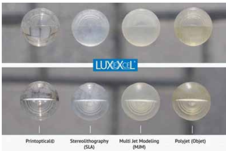
Figure 44: Results of Luxexcel's patented Printoptical technology in comparison to other AM technologies
