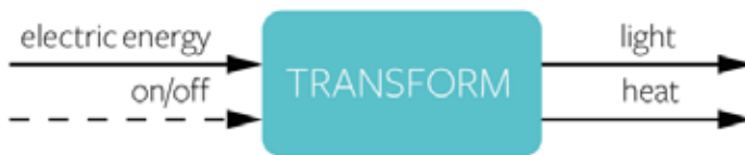
Figure 61. Black Box analysis of a LED Luminaire
