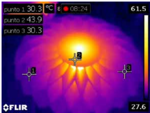
Figure 96 (a): Thermal image of the lamp with diffuser after 8 minutes and 24 seconds.
