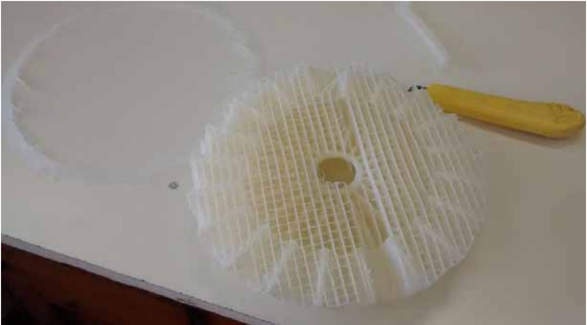
Figure 85: Removing the brim and the supports
