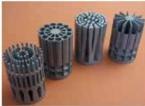
Figure 36: Heat sinks manufactured by DMLS
