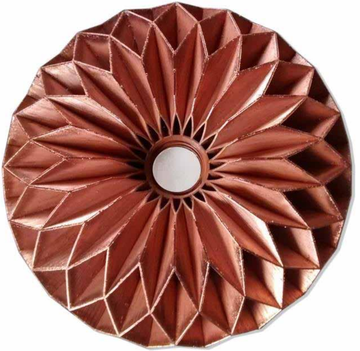
Figure 90: Arista body after copper plating
