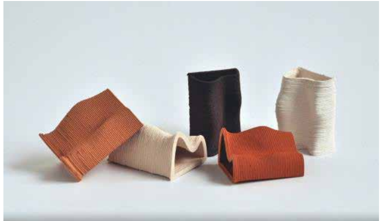
Figure 56: Clay printed parts by +Lab, Politecnico di Milano
