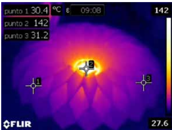
Figure 96 (b): Thermal image of the lamp without diffuser after 9 minutes and 08 seconds.
