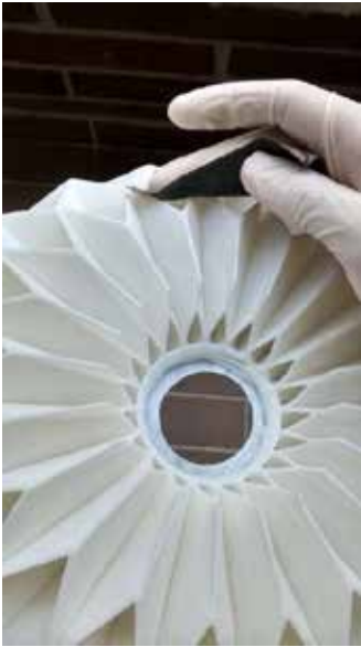
Figure 102: Sanding the edges of Arista V2
