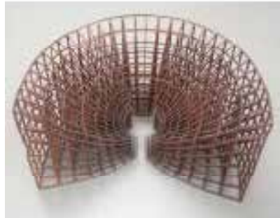
Figure 42: Custom nylon and copper plated heat sink.
