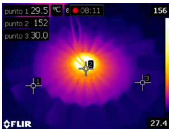
Figure 96 (c): Thermal image of the back of the lamp after 8 minutes and 11 seconds. Point 2, in the aluminum disc directly below the LED, shows a temperature of 152°C, which exceeds the LED's safe temperature limit of 150°C max.
