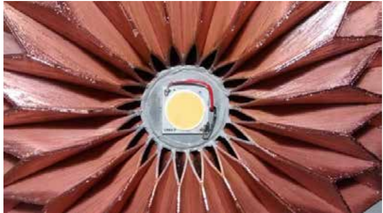
Figure 91: Detail of the assembly between the COB, the aluminum heat sink and copper body
