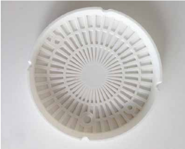
Figure 104: Driver compartment printed in white PLA
