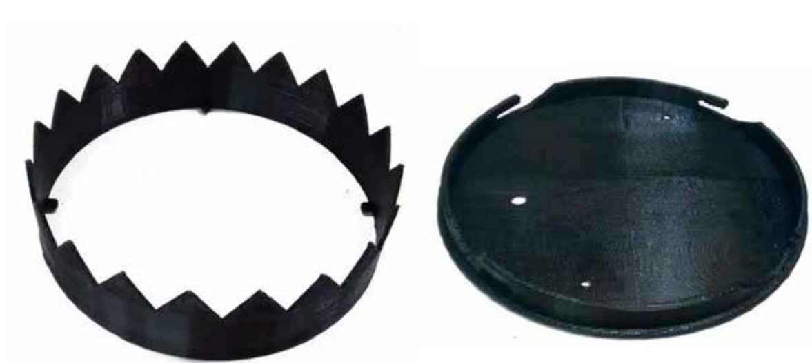
Figure 86: Crown-shaped ring and base plate prints
