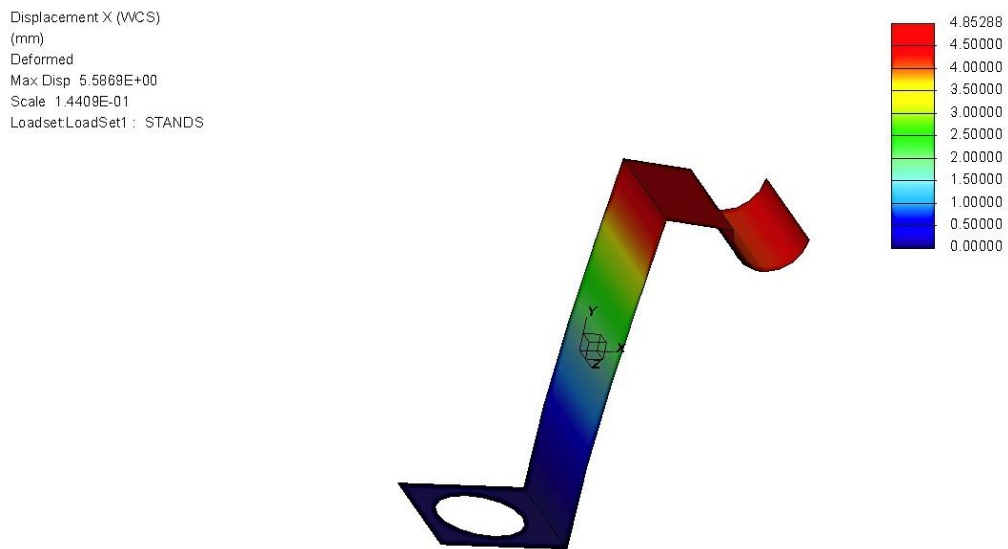
Figure 2-16 Displacement in x direction
