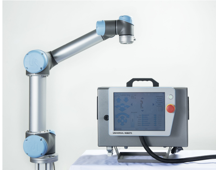
Figure 6.16: UR5 robot and its Polyscope control panel.
