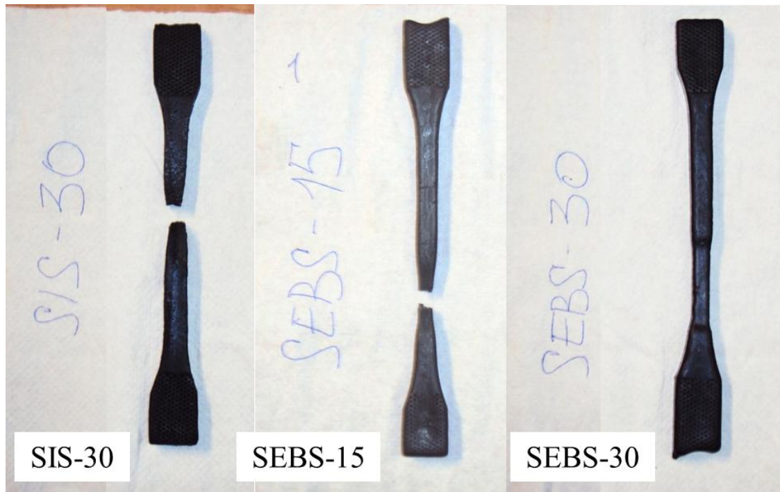
Figure 3–26 Samples of each tested formulation after tensile tests were performed. SIS30, SEBS15, SEBS30 respectively
