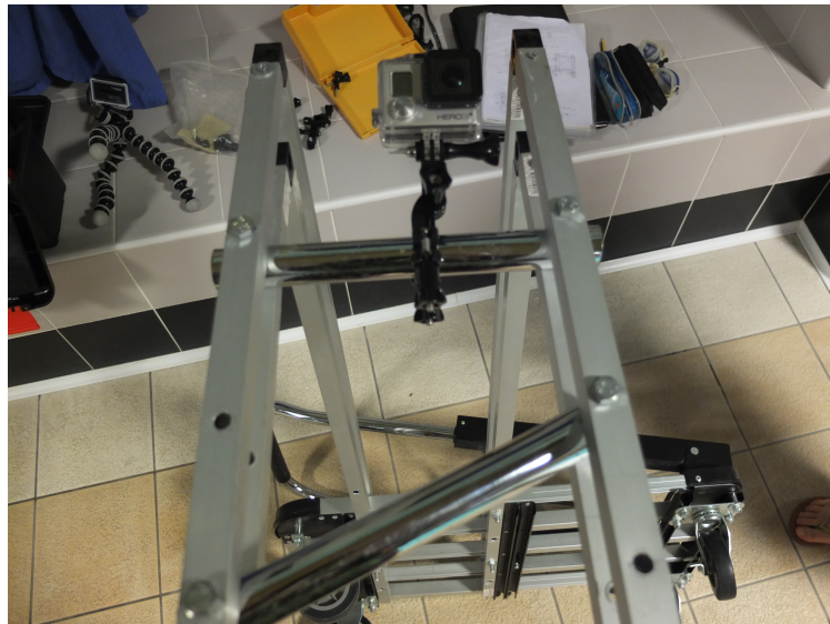
Figura 3.8: Positioning of the cam on the round tube with the GoPro mount.
