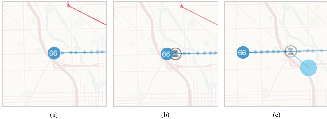
Figure 4: The sequence of figures illustrates how transfers to other vehicles are highlighted. Figure (a) represents the situation before the transfer station. Figure (b) shows that when the vehicle passes by a station where there is at least one possible transfer, a representative marker pops up and fades out as the connecting trip passes by (figure (c))
