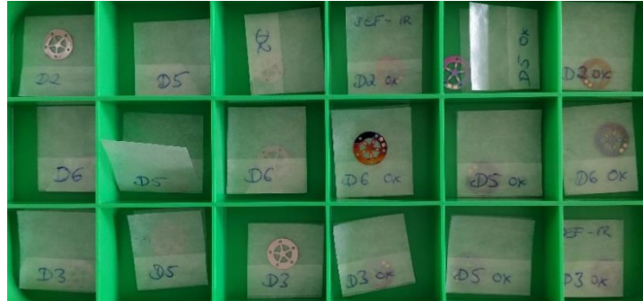
Figure 102 Prototypes with and without microheaters
