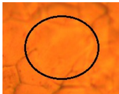
Fig. 3.13: darker areas on the 6 min CVD Copper sample
