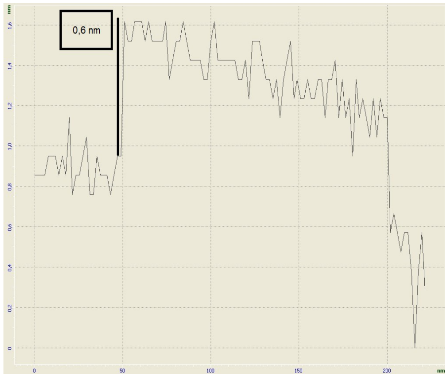
Fig. 3.42: qualitative evaluation of the graphene layers thickness
