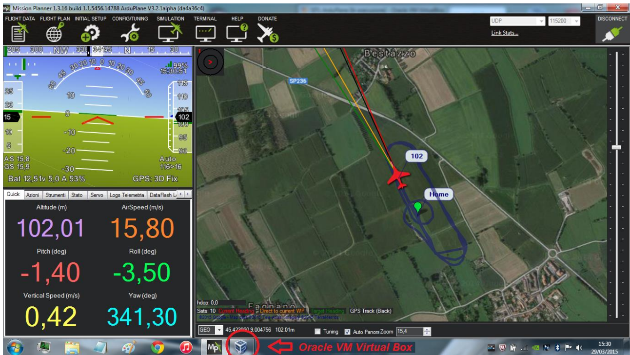
Figure 5.10 – SITL simulation run on the real flight tests local field map
