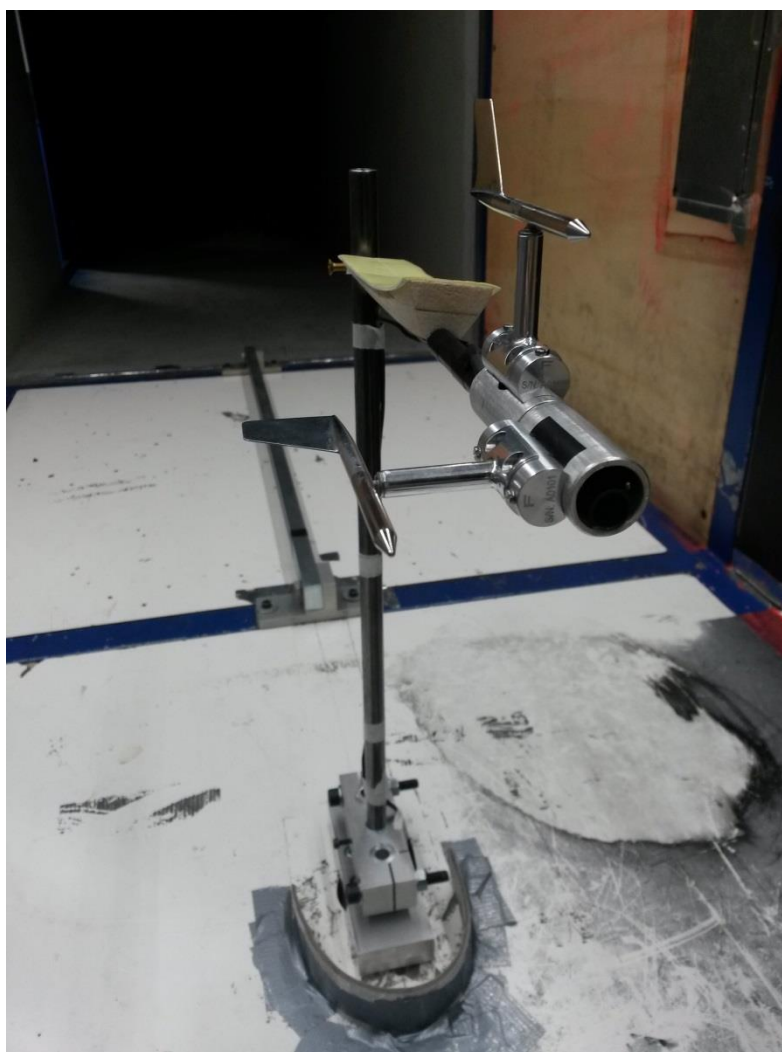
Figure 4.34 – AOA and AOS sensors off wing
