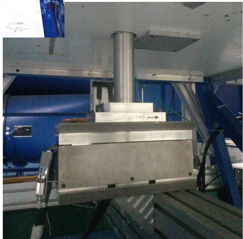
Figure 4.5 – The wing support connected to the 3-axis balance underneath the floor of the wind tunnel test chamber
