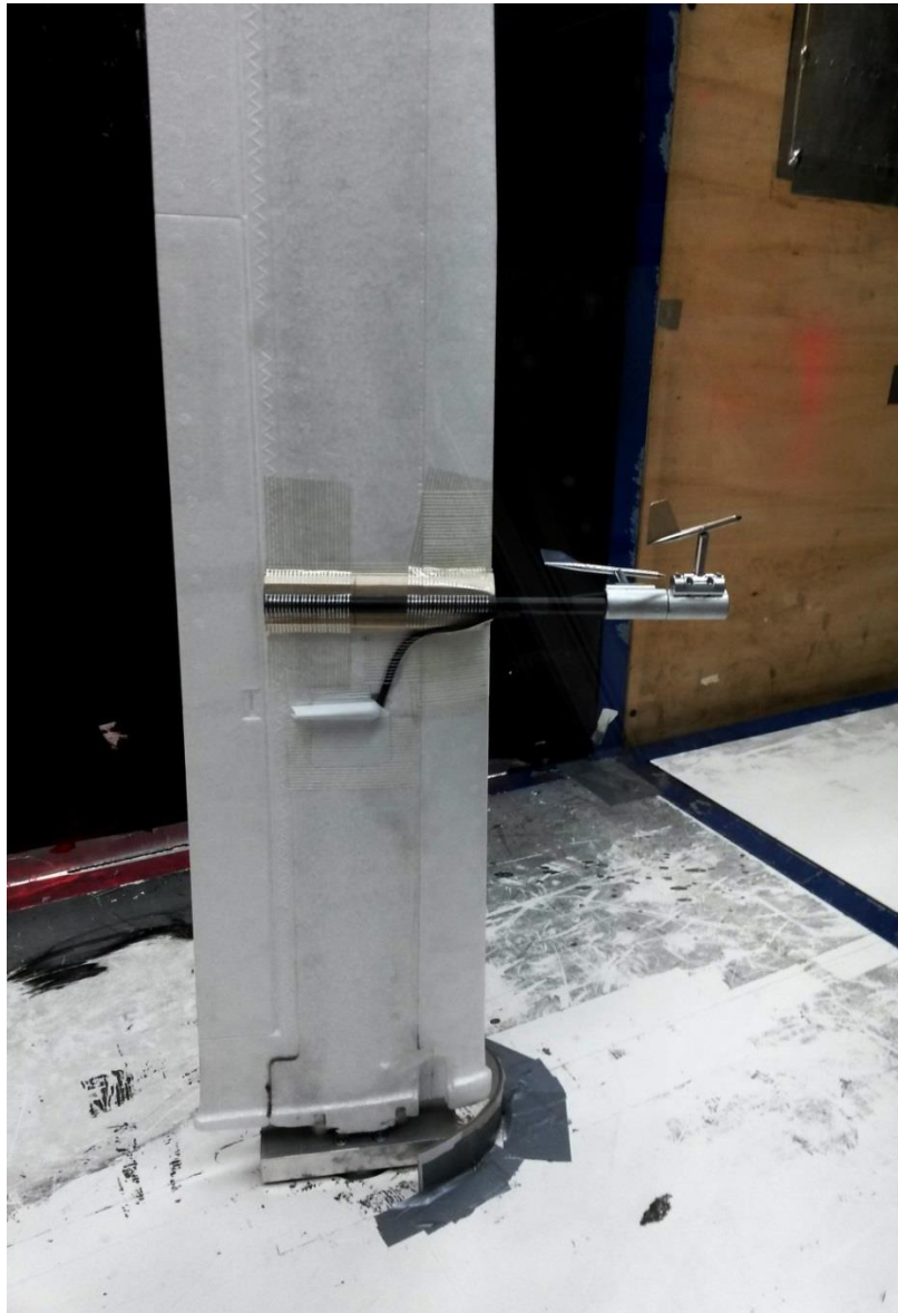
Figure 4.33 – Particular of the wind tunnel model with the AOA and AOS sensors installed
