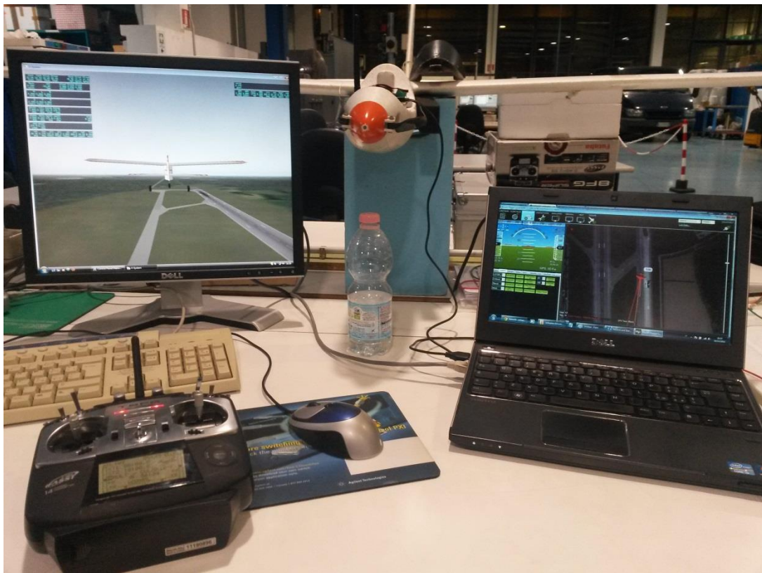
Figure 5.8 – The HIL simulation running on the two computers
