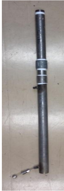
Fig. 3.14 Stainless steel venting pipe.
