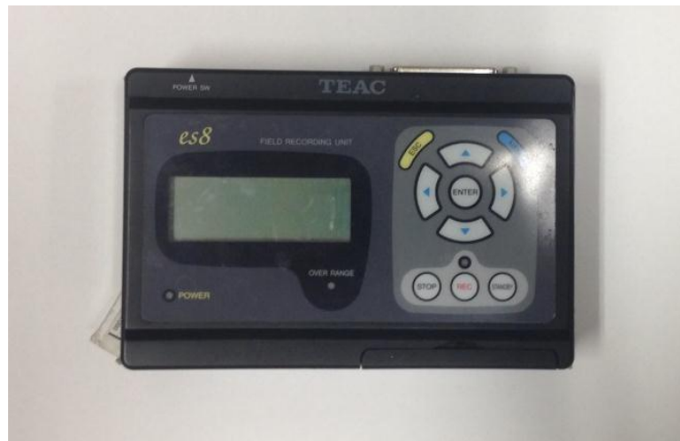
Fig. 3.21 TEAC es8 data acquisition system.
