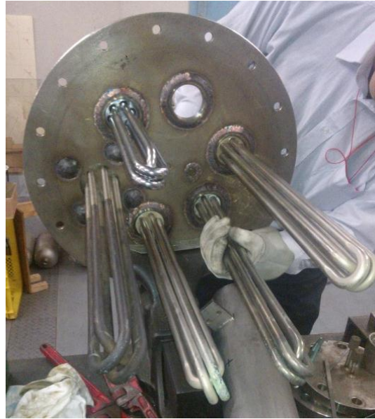
Fig. 3.5 Picture of the electrical heaters connected to the lower plate of the main tank.
