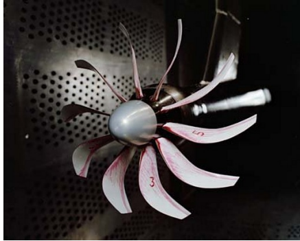
Figure 4: Experimental Setup of SR-5 propeller [30]
