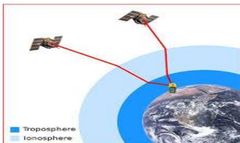
Fig. 3. 5: Tropospheric and ionospheric delays (source: http://www.brighthub.com/electronics/gps/articles/111933.aspx ).
