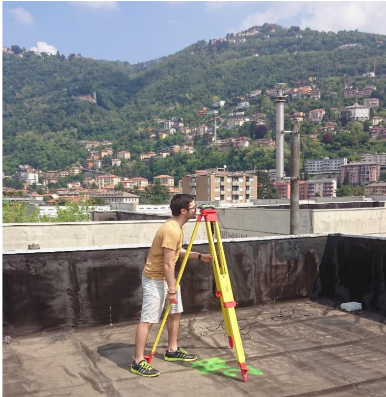
Fig. 5. 3: Centring and levelling procedure.
