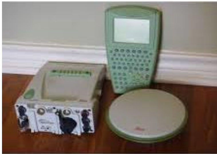
Fig. 3. 1: Leica GRX1200 and AX1202 GG antenna.
