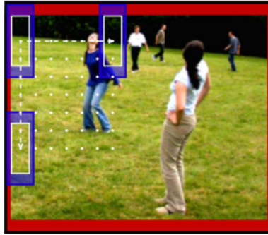
Figure 3.2: Sliding window running over the image allowing for the detection of pedestrians. The padding area of the detection window is marked with a blue shading.
