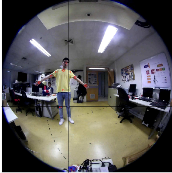
Figure 5.2: Example of Kinect auto calibration where the user to click on points on the image corresponding to Kinect skeleton joints, in a given order. These point coordinates will be later used to solve the optimization problem.
