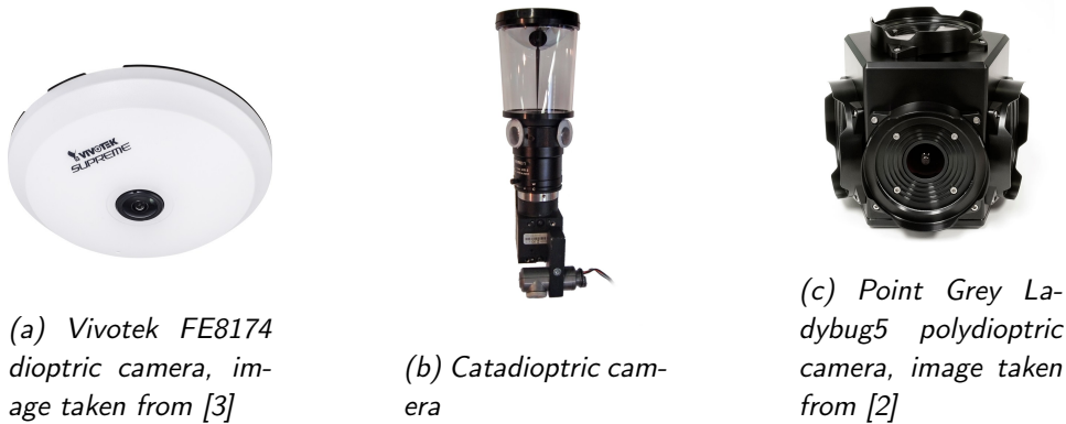
Figure 2.3: Examples of omnidirectional cameras. Dioptic cameras offer a field of view of 180^\circ over the vertical and horizontal plane. Catadioptric cameras offer a 360^\circ field of view over the horizontal plane but must be placed on top of the robot at a reasonable height. Polydioptric cameras are the only ones able to acquire the entire sphere around the camera.
