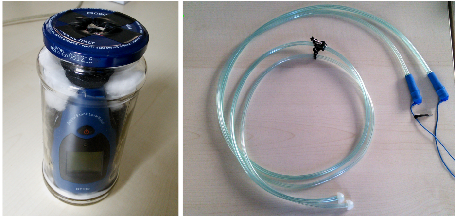
Figure 3.7: On the left image there is the sound level meter placed inside of a glass jar padded completely with a sponge and cotton used to measure the in-ear headphones SPL. On the right image there are the in-ear headphones designed with the PVC (PolyVinyl Chloride) tube.
