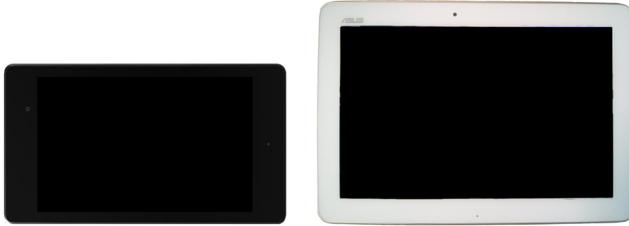
Figure 3.6: Host devices used in the auditory BCI system. On the left: Asus Nexus 7 2013 with Android™ Lollipop 5.1.1 (7" LED Backlight WUXGA 1920x1200 Screen IPS Panel). On the right: ASUS Transformer Pad with Android™ KitKat 4.4.2 (10.1" LED Backlight WXGA 1280x800 Screen IPS panel).
