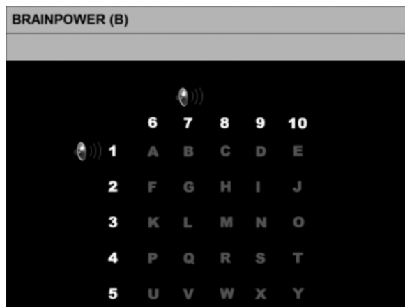
Figure 2.26: The 5x5 visual support matrix for the auditory ERP speller. The numbers surrounding the matrix aimed at facilitating finding the target coordinates. Each number corresponded to an auditory stimulus. For instance, to select the letter "B" the user was required to focus attention on auditory stimulus "one" during the first interval of the trial and on auditory stimulus "seven" during the second interval of the trial.
