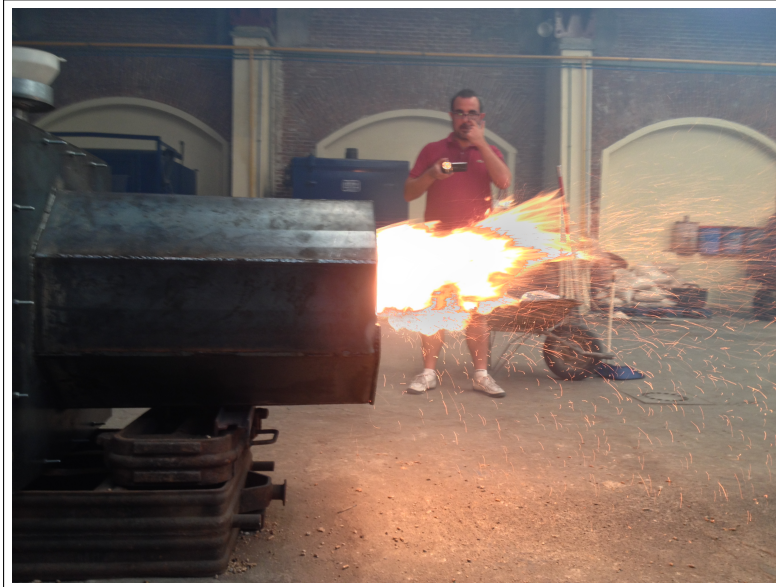
Figure 4.8: Actual burner in operation
