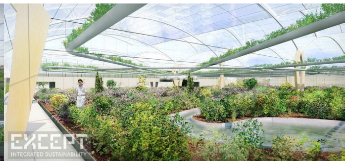
Figure 2.9: A 3D simulation of what a Polydome system could look like. In the image the hydroponics system is suspended over the temperate zone. [28]
