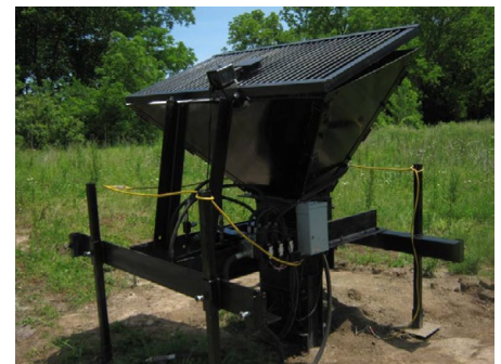
Figure 2.23 : Compressed earth block press. Image source: http://opensourceecology.org/wiki/CEB_Press
