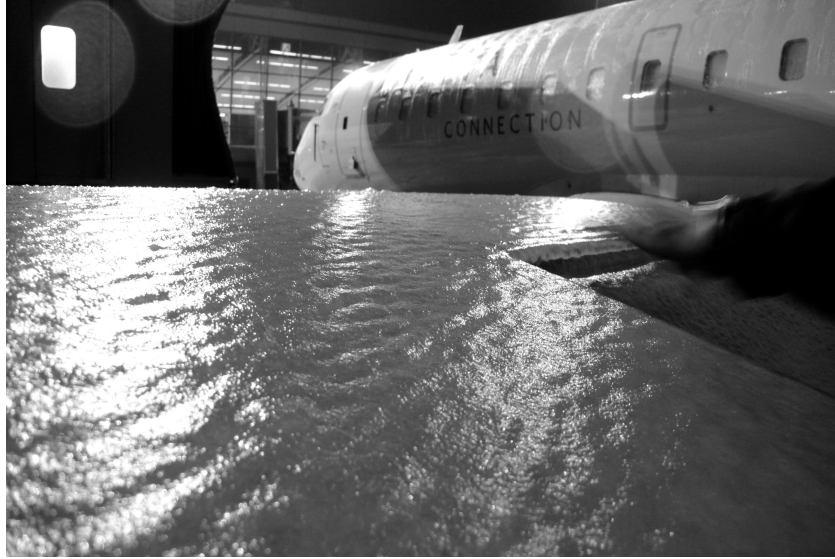
Figure 1.2: An example of the effects of the freezing rain over a wing. The ice covers the entire surface of the wing. Image taken from Ref. [2].
