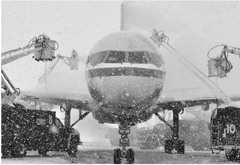
Figure 1.9: Example of the application of the anti-icing chemicals. Image taken from Ref. [6].
