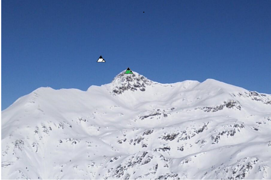
Figure 3.8: Compass Matching Result: the white marker represents the peak estimate only based on embedded sensors. The green marker is the estimate obtained from the groundtruth.
