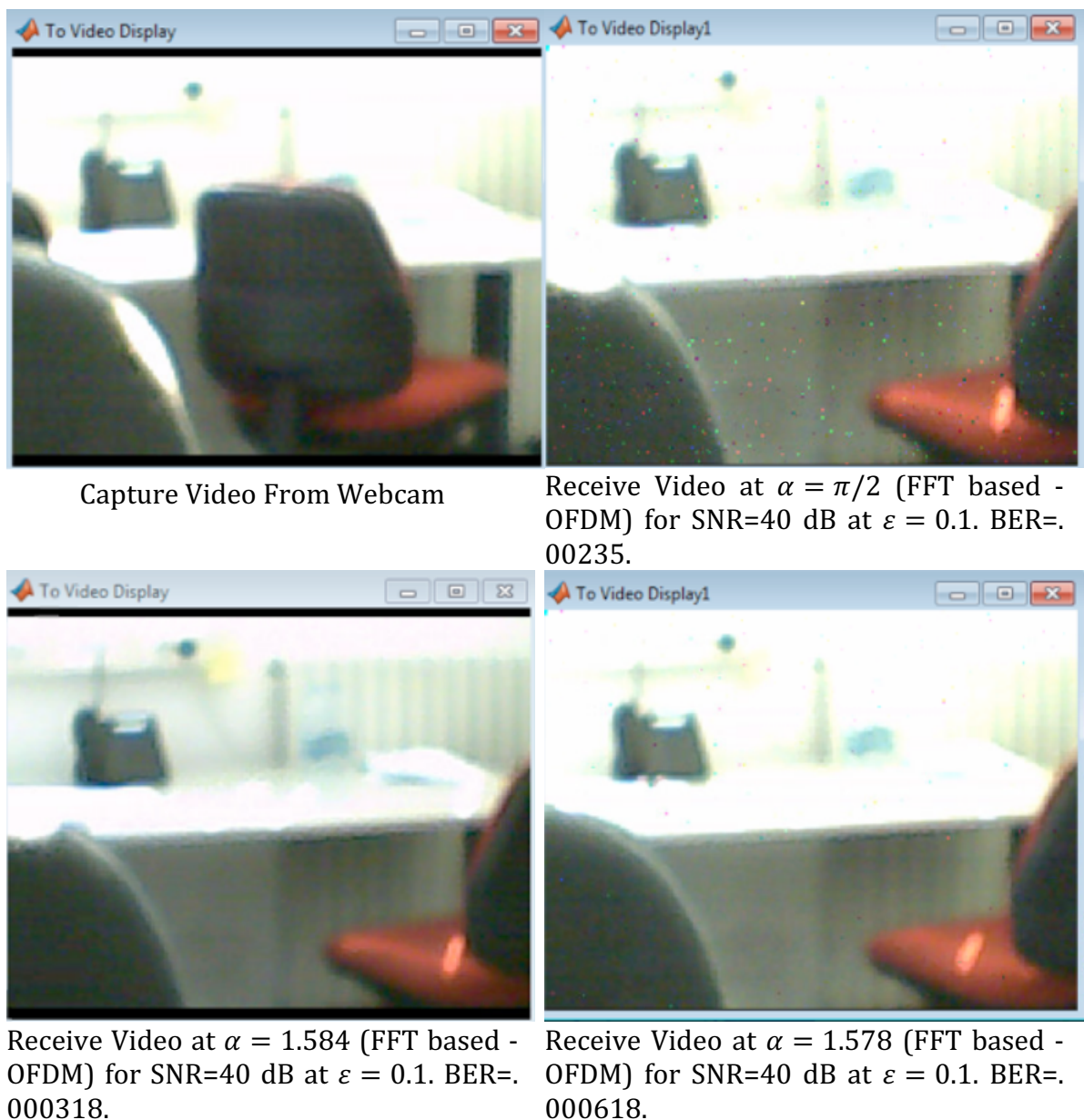
Fig. 4.5.1 Example of captured and reproduced video signals in case of an FrFT based- system and an FFT based- system.
